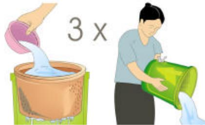
Doing one of the above two steps will flush the clay smell and color from the ceramic pot. You only need to do one of the above steps, it is not necessary to do both.
