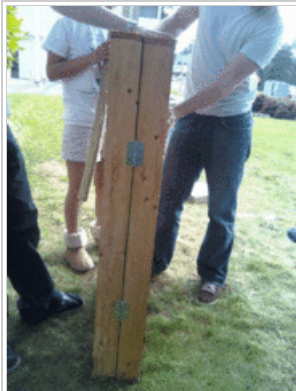
Figure 3: Side view of the frame with hinges.
