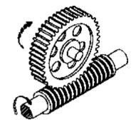
Worm Gears Teeth are at an angle and curved There is axial thrust **APPLICATION - Gear box.**
