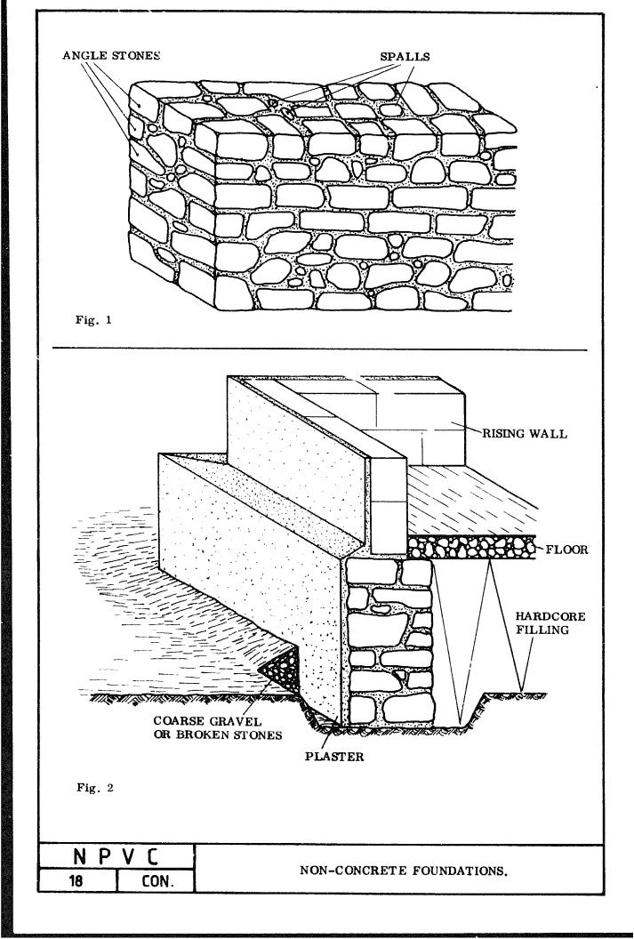
used: not only foundations but also footings, plinths and even rising walls were made out of stones. Due to the increased use of cement worldwide, and the improved concrete technology, stone masonry became uneconomical to build with because it takes more time and labour. Eventually the use of some of these types of masonry disappeared.
