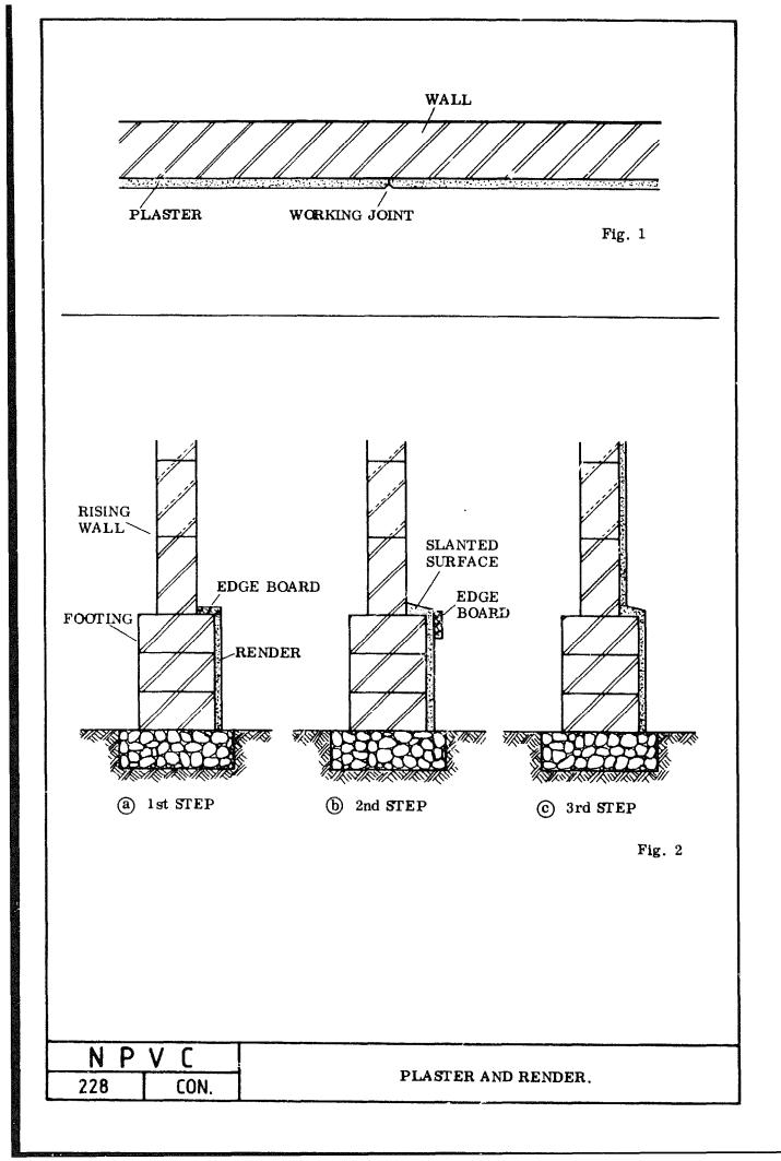
The plaster or render is generally applied in a single layer on top of the spatterdash, or else directly on the blockwork surface. This layer will be 15 to 20 mm thick.
