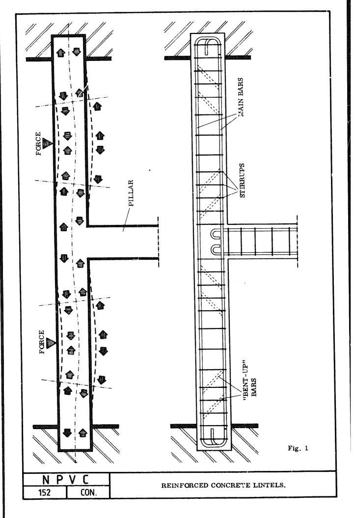
On the left is a drawing of a reinforcement system for a continuous beam; this might occur for example in an eave beam supported by a reinforced pillar (Fig. 1).
