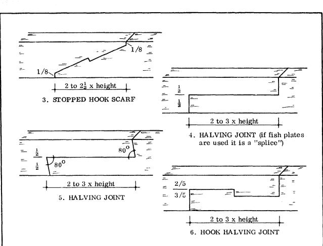
Joints 1 - 6 are normally used for joining rafters, tie beams or purlins in the length. They can be used with one or two fish plates.
