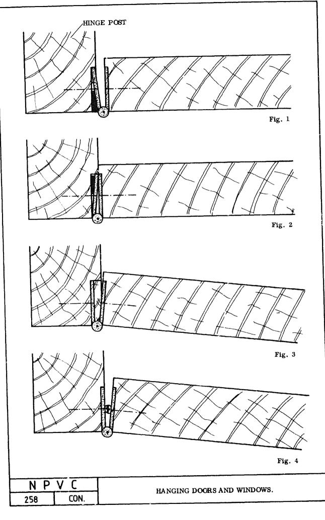
k. Place the door in position and fix it to the door post with one screw in each leaf of the hinges. Close and open the door several times to see if it works smoothly. Notice in particular whether the door closes completely and does not scrape either post. It should stay closed by itself.
