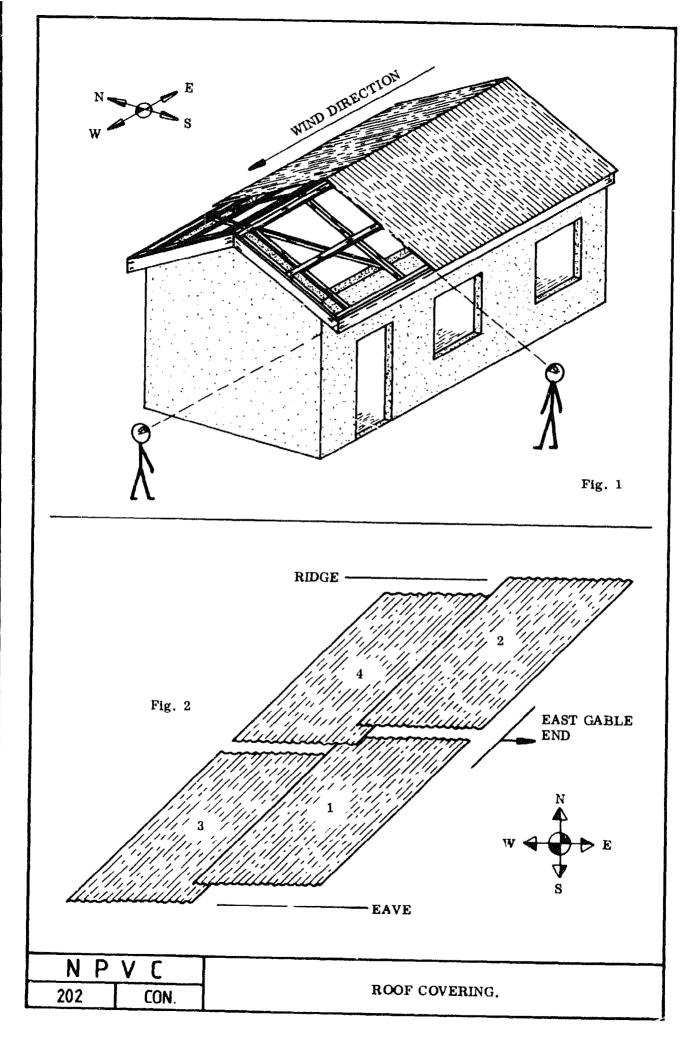
The helpers can also check from both sides of the roof to see if the corrugations match at the ridge line (Fig. 1).
