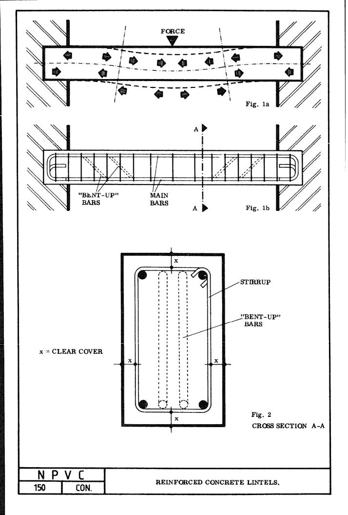
The longer reinforced beam or lintel shown here in Figs. 1a and 1b is reinforced with main bars on the top and bottom.
