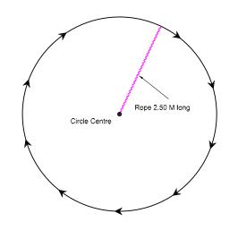
(2) Marking the Internal Diameter
