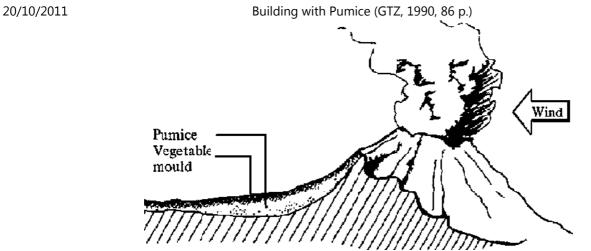
Figure 6: Pumice deposits on the downwind side of a volcano
