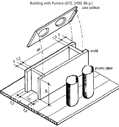
Figure 31: Wooden mold for two-cavity blocks
