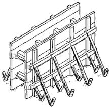
Figure 50: Wooden formwork for in-situ pumice-concrete walls
