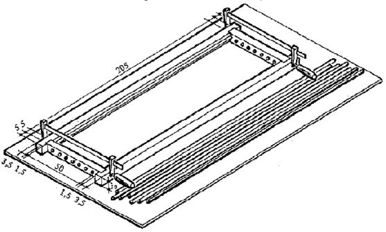
Figure 39: Mold for hollow-core planks
