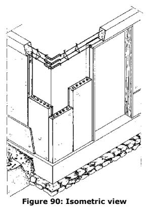
4.5.2 Hollow-core planks 30  $\times$  205  $\times$  12 cm
