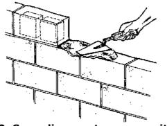
Figure 32: Spreading mortar on a cavity block
