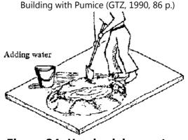
Figure 24: Hand-mixing system
