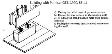
Figure 33: Forming pumice-concrete two-cavity blocks
