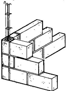
Figure 45: Masonry corner with channel block serving as support fromwork
