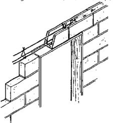
Figure 43: Channel form block in a tie-beam configuration
