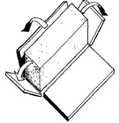
Figure 26: Immediate removal of forms possible
