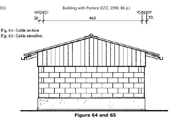
The roof can be covered with clay roofing tiles, corrugated asbestos, corrugated metal, reed or palm fronds.
