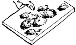
Figure 21: Proper moisture content of pumice-concrete
