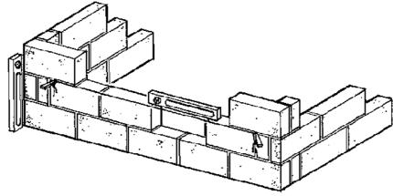
Figure 57: Setting up brick walls
