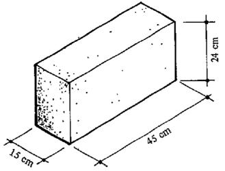
Figure 27: Pumice-concrete solid brick.
