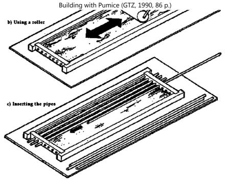
Figure 40: Forming pumice-concrete hollow-core planks
