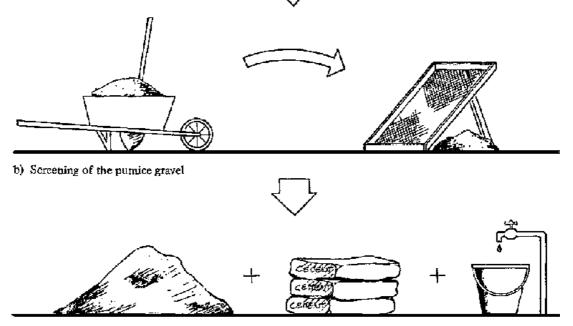
c) Materials for pumice concrete: pumice gravel, cement, water
