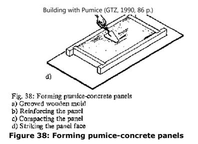
The panel-making area must be absolutely level. Each panel should have its own support made of smooth sheet-metal or wood. If nothing else is available, smooth paper or plastic sheeting can be laid out under each mold/panel, as long as the ground is perfectly level.
