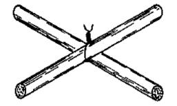
Fig. 2b BINDING OF CROSSING BARS
