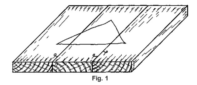
The boards that will be joined must first be marked. Lay the boards out in the desired position and mark them with a triangular mark over all the boards (Fig. 1). The triangle should point upwards. This mark will help us to keep in mind the position of each board during the steps that follow.
