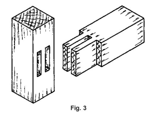
The sequence of operations is almost the same as for the common mortice and tenon joint, with the only difference being that two mortices and tenons have to be marked and cut instead of only one.
