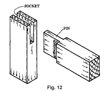
The pin is constructed like the tenon in the sequence of operations for the mortice and tenon joint for frame-like constructions, pages 118 to 120.
