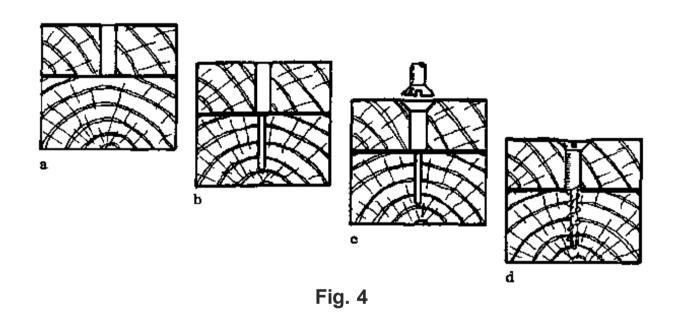
Use a screwdriver with the correct tip only. If the screw turns too hard, the hole may be too small or not deep enough. Remove the screw and find out what the problem is so it can be corrected, otherwise the screw may break or split the board.
