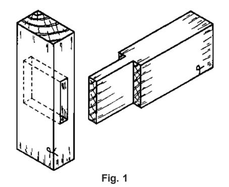
The sequence of operations to construct a mortice and tenon joint for frame-like constructions is almost the same as for box-like constructions. Of the four types of mortice and tenon joints mentioned in this chapter, we will only go into detail about the construction of one of them, the common mortice and tenon. No new tools will be needed.
