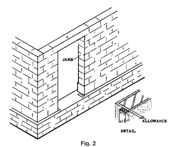
A jamb is the portion of wall, or wall face, at the side of an opening. The jambs are built a little wider than the outside measurement of the frame (Fig. 2) so that the frame can fit into the wall opening.
