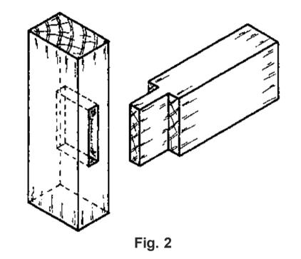
At times a combination of the haunched and stub tenons is required. This is called a haunched stub mortice and tenon joint.
