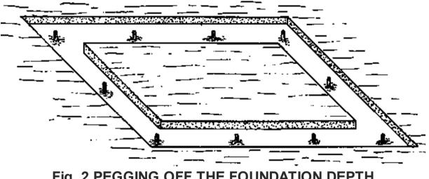
Fig. 2 PEGGING OFF THE FOUNDATION DEPTH
