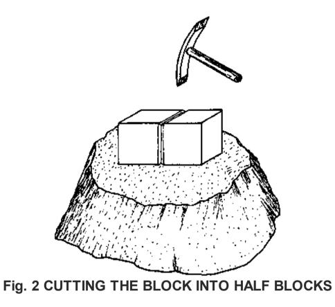
Trim the resultant rough header faces, if necessary, with the edge of your trowel blade (for landcrete blocks). When cutting sandcrete blocks, you should use the block scutch for trimming (Fig. 3).
