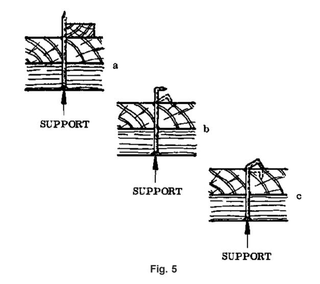
The head of the nail should be supported during clenching to keen it from being nusbed out again file:///D:/cd3wddvd/crystal\_A6/construction/stuff2.htm
