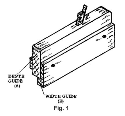
One wooden piece is fixed on the sole of the plane (B) at the standard width for rebates and another piece is fixed on the side of the plane (A) and can be moved up or down to adjust the depth of the rebate. The width can also be adjusted, by using a wider or narrower wood guide (Fig. 2).
