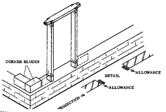
If for some reason the door frames are to be installed later, the jambs of the openings (Fig. 2) are built up as described in the chapter on stopped ends, page 22.
