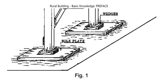
Formwork is made of wood or metal and consists of two structural parts: the shuttering and the strutting.
