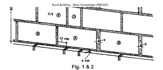
The second course of the T-junction begins with the full block of the inside wall that is bonded into the outside wall (Figs. 1 & 2, block D). This is followed by a 3/4 block (Fig. 2, block E) on the same side of the header where the stretcher (block A) below projects by 12 cm. Continue with full blocks in all three directions.
