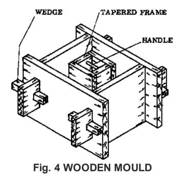
After the pier is built, the anchoring bar is inserted in the hole and the remaining space is filled up with mortar or concrete.
