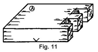
Step 5. Assembling the joint
