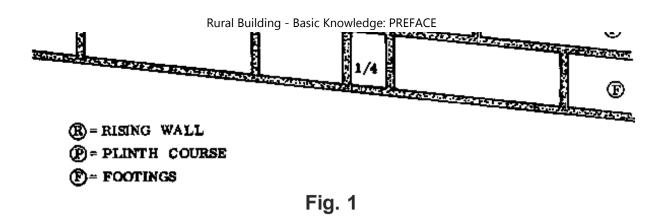
The only difference is that the first two cross joints in the inside wall are widened to 4 cm each, in order to maintain the half-block bond in relation to the footings.
