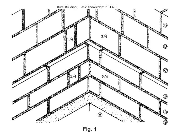
Again, it is possible to maintain the half-block bond between the footings and the plinth course in wall I, as described on the previous pages. The bonding of the plinth course is a repetition of the bonding of the second footing course.
