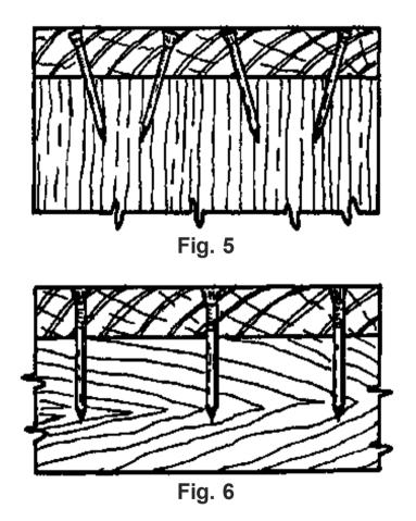
If possible the nails should be inserted at right angles to the force that will be applied to the piece; so that any force tends to shear off the nail rather than pull it out.
