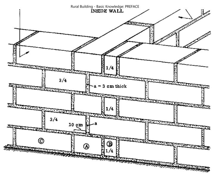
Fig. 1 & 2 COMBINED SECTION OF OUTSIDE WALL AND VIEW OF INSIDE WALL
