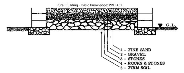
Fig. 3 HARDCORE FILLING
