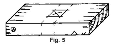
If the marking gauge has two pins, set each at its correct measurement and mark both lines at once. If not, mark with the first setting on all the members, then change the setting and mark the other file:///D:/cd3wddvd/crystal\_A6/construction/stuff2.htm measurement on all the members.
