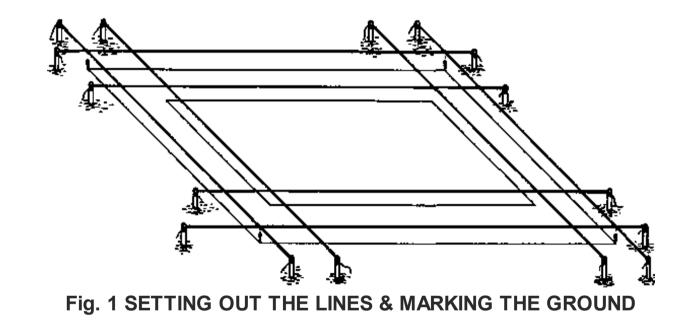
These marks will be needed until the plinth course is completed, so they must be relatively durable, so that they remain accurate for a longer period and are not destroyed by rain or other influences.
