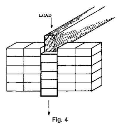
In order to make the wall stronger in itself and able to distribute loads properly, the Rural Builder applies the so-called half-block bond.
