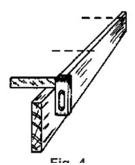
When all these tests have been performed with satisfactory results, the board will be straight and true in all directions and it is ready to be used in a project.
