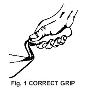
The amount of mortar picked up from the headpan will depend on the nature of the job, but for the trainee it is advisable to pick up a sufficient amount to lay one training block, i.e. a heaped trowel. Later, when working with the common big blocks, it will become necessary to pick up two trowelfuls of mortar.
