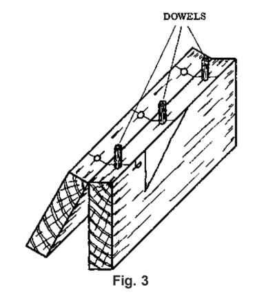
The holes should be about as deep as the boards are thick, and they should be slightly countersunk (see Fastening with Screws, page 96).
