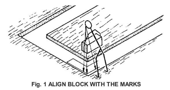
Use the straight edge with gauge marks to ensure that the block is laid at the correct height. Hold the straight edge vertically against the block; the top edge of the block should correspond to the gauge mark (Fig. 2).
