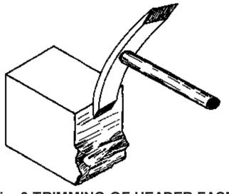
Fig. 3 TRIMMING OF HEADER FACE
