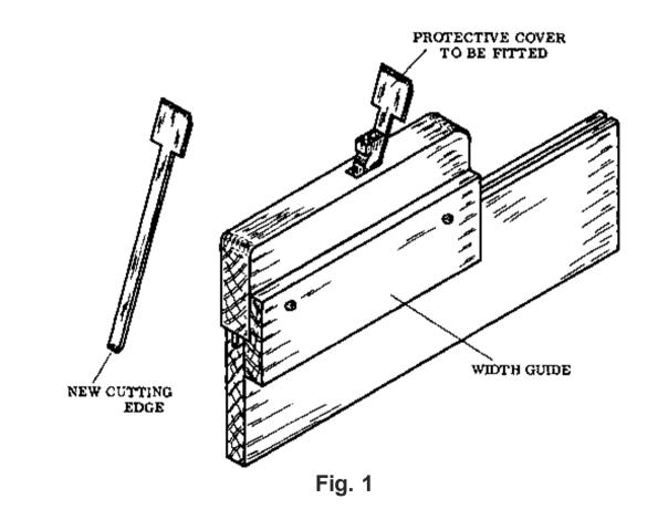
To do this, grind and sharpen the narrow end of the rebate plane cutting iron to make a cutting edge. Grind the sides of the iron to the size of the most commonly used tongue, which is 6 mm plywood. The sides should be slightly bevelled to ensure free movement in the groove. When the iron is fitted into the plane it is adjusted so that the cutting edge projects out of the sole by exactly the required depth of the groove.
