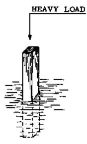
Fig. 2 POLE GIVES WAY AND SINKS DOWN
