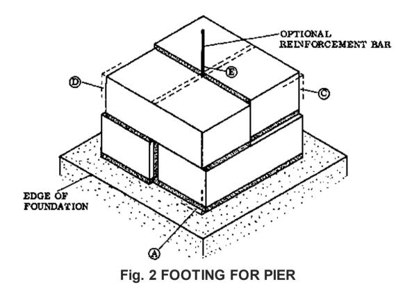
This is done to maintain a square shape of 48 cm by 48 cm, since the width of the two blocks plus a joint is 48 cm, while the length of each block is only 46 cm. Since the courses cross each other, a reinforcement bar for anchorage could be built-in between the cross joints (Fig. 2, E).
