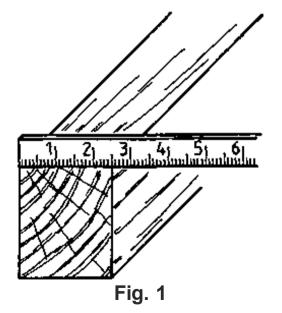
When the end of the rule has become worn and inexact, you can still get an exact measurement. Place the 1 cm mark of the ruler at the first point and read at the second point. The true measurement is that reading minus 1 cm. For example, the measurement in Fig. 2 is: 3,5 cm minus 1 cm equals 2,5 cm.
