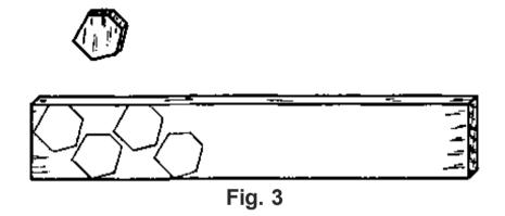
The template is used by placing it on the material to be marked and holding it firmly in place while drawing around it.
