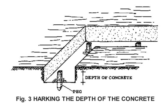
If the exposed heights of the levelled pegs are not equal, that means the bottom of the trench is not level. The uneven spots have to be levelled by taking out some soil, until all the pegs project equally.
