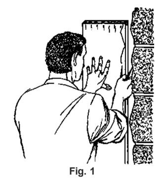
As one leg of the compass moves along the wall, the other leg will mark on the board an exact copy of the irregularities of the wall surface. The legs of the compass have to be set apart by a distance a little greater than the width of the biggest gap between the wall and the board.
