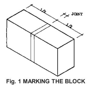
Before cutting a block, mark the required size around all the faces. To prevent mistakes and to speed up the work, use a block gauge (see Rural Building Reference Book, Tools, page 12). Position the appropriate setting of the gauge against the block, then mark off the measurements on the block face using a pencil or a nail.
