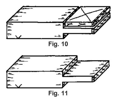
Step 5. Assembling the joint
