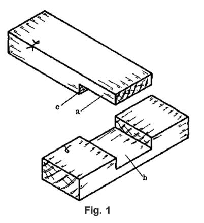
The pin is half the thickness of the timber, and the depth of the socket equals the thickness of the pin. The shoulder of the pin (c) fits against the face edge of the socket (Fig. 1).
