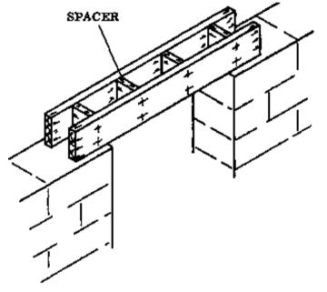
Fig. 2 WIDE BUILT-UP WOODEN LINTEL
