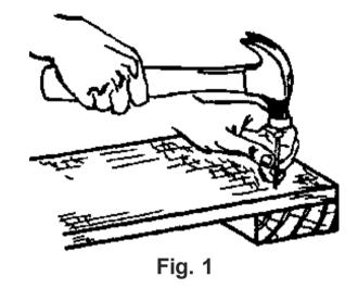
After the nail is well started, drive it in with firm blows. Hold the handle of the hammer near the end and strike the nailhead straight.
