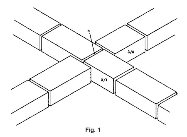
The two 3/4 blocks of the first course are arranged so that they are at right angles to each other. One of the 3/4 blocks always starts from the middle of the crossing wall while the other is placed on either the right or left side of it. This is followed in all four directions by full blocks (Fig. 1).
