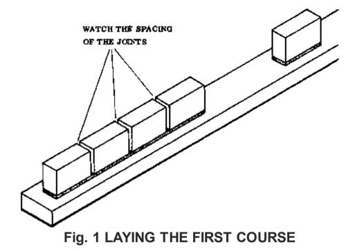
Their height is adjusted by placing the straight edge on top and pressing the blocks down until the top surfaces of all the blocks touch the straight edge equally, along their whole length.
