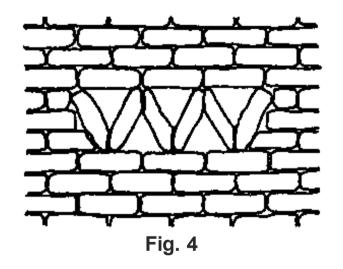
The wider an opening becomes, the more difficult it is to bridge. Builders from many parts of the world eventually learned that if the blockwork remains closed above an opening, both sides of the wall will support each other, maintaining stability. This knowledge was often applied not only to bridge openings but also to construct roofs. The technique was to let each course overlap the one below until the blockwork met at the top and the two sides bonded into each other (Fig. 5).
