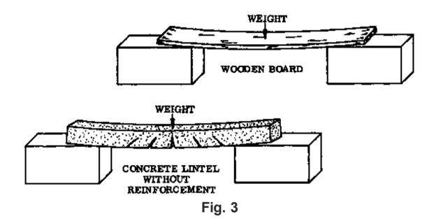
To prevent this, reinforcement bars are embedded in the concrete if the lintel is expected to receive tensile stresses. The combination of concrete and steel does the job where one of them alone would not work: the concrete resists all pressure while the embedded steel resists all stresses.
