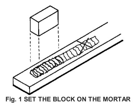
If the bed has been spread correctly, only a few taps with the handle of the trowel will be needed to adjust the height of the block. The height is checked by comparing the height of the block with the gauge marks on the straight edge (Fig. 2).
