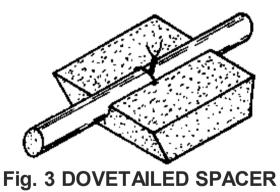
There must also be spacers on the sides of the cage, to hold the stirrups away from the side boards of the shuttering.
