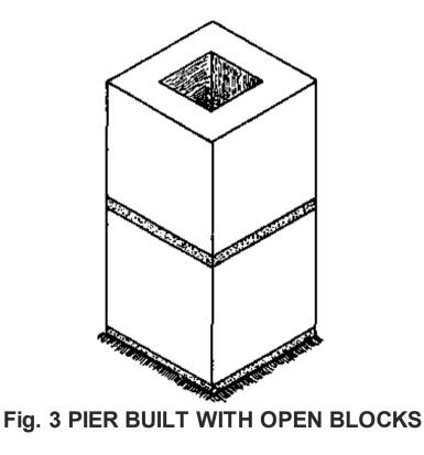
Open blocks are made by casting mortar between two frames (Fig. 4). The bigger frame is made similarly to the wooden mould described in the Reference Book, Tools section, page 29. The smaller frame is tapered and has a handle to make it easier to remove from the block.
