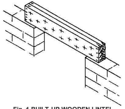
Fig. 1 BUILT-UP WOODEN LINTEL
