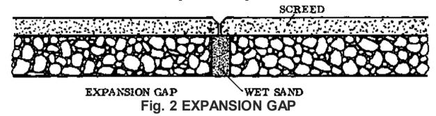
The expansion gap allows the floor to expand and contract with the temperature changes without forming cracks. Expansion occurs when the floor is heated by the sun during the day, and shrinkage occurs at night when it cools down. Floors exposed to the sun should be divided into bays of no more
