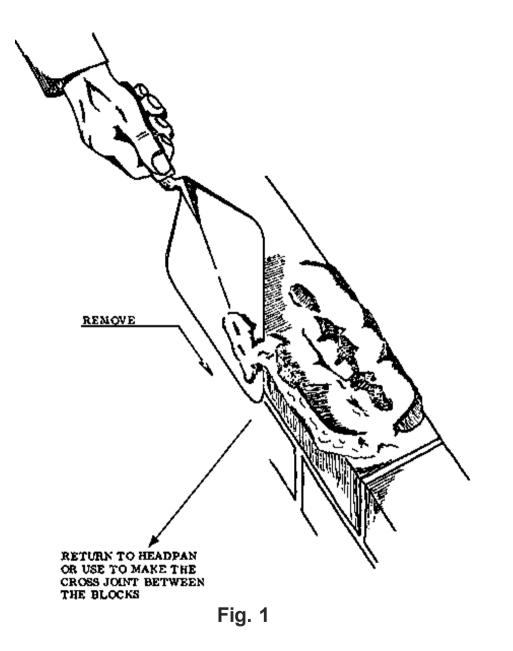
The surplus mortar recovered on the trowel is usually taken to form the cross joint between the last laid block and the previous one, or it is returned to the headpan.
