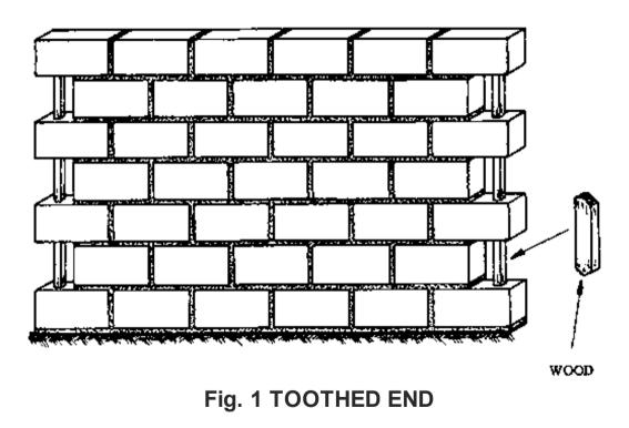
This block must be exactly above the first block of the first course. To ensure this, hold the spirit level against both header faces and make any necessary corrections. It is not necessary to level the top face if the stretcher and header faces have been plumbed.
