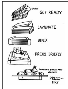
Figure 2: Laminating - work quickly, race-the-stretch
