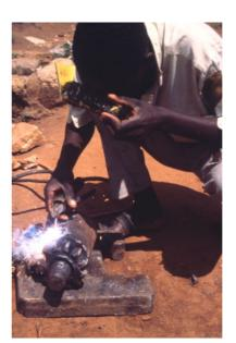
Figure 1: Kennedy Otieno repairing a sugar crusher for jaggery production. Migori, Kenya Photo credit: Practical Action/Morris Keyonzo
