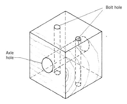
Figure 1: One-piece block bearing
