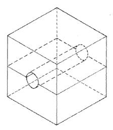
Figure 2: Split-block bearing
