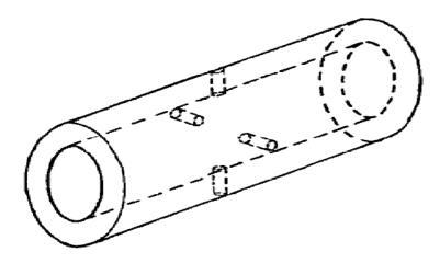
Figure 3: Bush bearing showing the four lubrication holes
