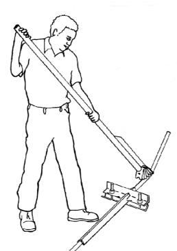
Operation of the pending tool is relatively easy. The pipe that you wish to create a bend in is placed in the clamp and the two nuts are tightened to ensure that the pipe does not slip. Once the pipe is clamped up the bending arm can be slipped onto the pipe and positioned appropriately. The long arm of the tool makes the job of bending the pipe easy.
