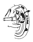
2. PUT A NEW RUBBER ONTO THE BOBBIN WINDER BY PUSHING IT GENTLY OVER THE EDGE AND INTO THE GROOVE.
