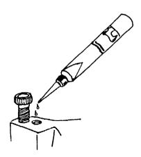
2. WHEN YOU HAVE PUT OIL IN ALL THE HOLES, TAKE OUT THE NEEDLE, AND RUN THE MACHINE VERY FAST FOR A FEW MINUTES SO THE OIL WILL SPREAD TO ALL THE PLACES IT IS NEEDED.
