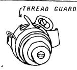
THE THREAD GUARD FOR THE TEN-SION REGULATOR IS A PART OF THE TENSION REGULATOR ITSELF. IT IS A BAR OR CURVED PIECE THAT STICKS OUT FROM ONE OF THE PIECES OF THE TENSION REGULATOR.
