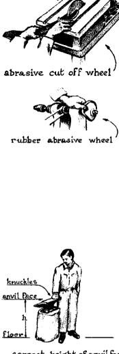
correct height of anvilface from Floor level
