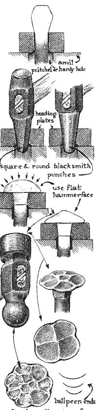
of various diameters for texturing steel surfaces
