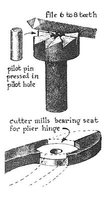
Now reduce speed to about 1000 rpm or less, and drill the pilot hole at that speed until the bo't head comes flush with the vise jaws. Raise the bolt head, stop the motor, and remove the drill, but keep the vise tightly clamped on the drill-press table.
