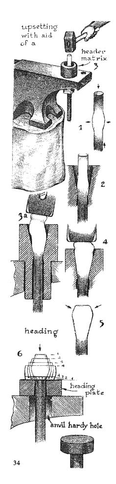
Once it is annealed, test the matrix with the file for hardness to make very sure it is soft enough for drilling.
