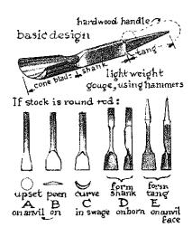
if stock is rectangular bar, its width is to be twice its thickness
