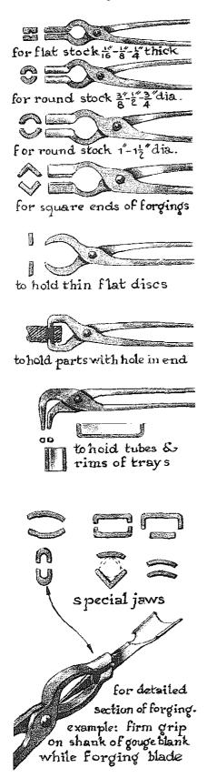
Specific workpieces demand different jaw shapes in the tongs used. The shapes shown here simply aim to give an idea of the kinds of stock different tongs are suitable to hold. For instance, the woodcarvinggouge blank shown required the narrow-slotted tongs to match the gouge's upright shank. These tongs can, of course, be used for other things as well.
