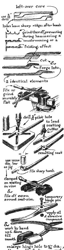
enlarge hinge hole to 5% dia., disassemble & temper each element separately: jaws a dark straw, hingeseats purple, handles pale blue.
