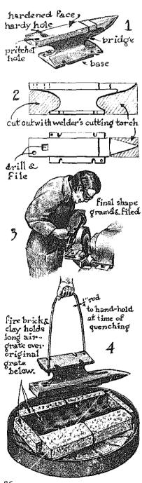
shallow tray with an inch of water to cool the anvil face. 50-gallen drum to line water ready to quench it. Also have ready a Before you start the for tempering the anvil, be sure to have a
