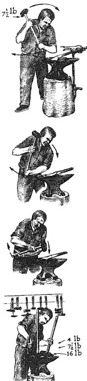
heavier sledges to be used on heavier anvils
