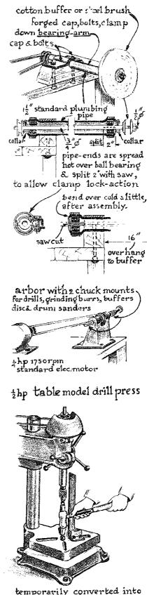
a woodworking lathe to turn tool handles.
