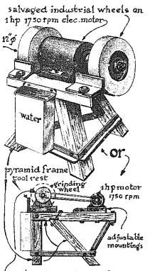
empty motor housing used as grinding wheel arbor.
