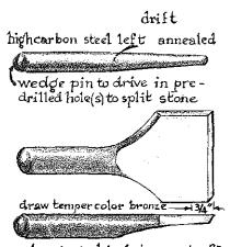
cleaving chisel to crack off segments along precut groove.
