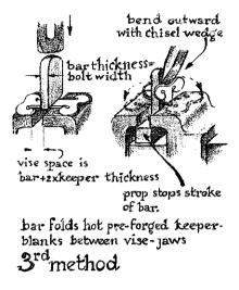
This die set can be placed free on the anvil face when you are using a set hammer. Press the set hammer down on the end of the jig, forcing the die down onto the hot keeper blank, before striking it with a 4-pound hammer.
