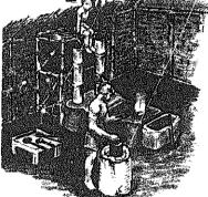
Fuel: teakwood charcoal anvil: broken shaft of sugar mill crusher, set in wood stump Forge: basind air ducts in clay quenching tub: hollowed out log shop: bambu structures clay Floor
