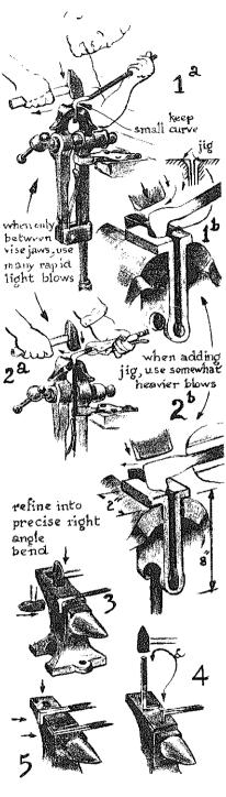
keep small inside curve until step 4 use vise-grippliers if tongs fail to hold firmly 3-4-5 sharpens all edges & aligns to 90° angles
