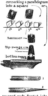
squared ends forged into tapered ends become 1½ to 2 times longer the correct position.) Just before the piece falls off with the final blow, gently strike it a little *outward* from the hardy edge, and it will be sheared off. This prevents striking the hardy and dulling it or damaging the hammer.
