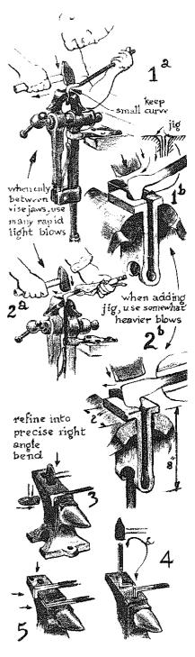
keep small inside curve until step 4 use vise-grip pliers if tongs fail to hold firmly 3-4-5 sharpens all edges & aligns to go° angles
