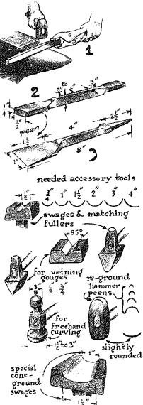
align blade with shank on anvil face by striking here heavier blows where blade is thickest, until bottom of shank & blade are straight shank. effective local blow with tip of fuller hold-fast anvil align blade with shank at each step close or open blade curve when needed during refining over horn important steps in forging conical blades of gouges in cylindrically ground swage grooves. when blade slants as shown strike hammer where cone contact runs parallel to swage groove
