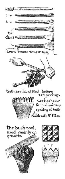
The most commonly used stonecarving tools are simple tools, little changed in design from earliest times. As a rule, stonecarving tools measure about 8 to 10 inches long, and 36 to 34 inch thick. All are made from high-carbon steel.
