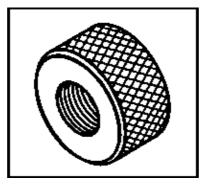
16 Cr Mn 5 (low-alloy steel, alloy constituents: 0.16% carbon, 1.25% chromium, less than 1% manganese, rest iron)
