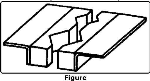
Steel sheet will be cut to size by long and straight sawing cuts; solid square steel will be sawn by mitre cuts (the required angle will be given by the instructor).
