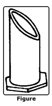
Light metal or steel sheets or tubes will be sawn to given dimensions to practise mitre cuts. After glueing, soldering or welding, these components can serve as containers for pins or scribers.
