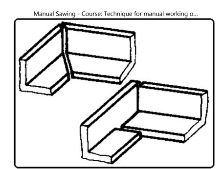
Straight and mitre cuts serve to practise the technique of joining angle steel to form a frame. Emphasis is to be laid on the peculiarities of straight and mitre cuts. Welded with the supports mentioned in instruction example 4.2., a frame for a table is produced which can be provided with an insert (of steel or wood) so as to form a table for putting down tools etc. in the workshop.
