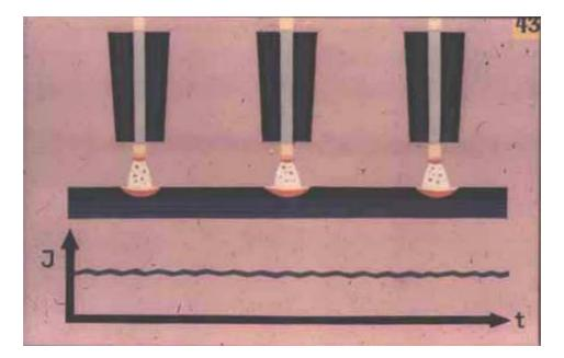
When using the high–current  $CO_2$  technique, transfer by the spray mode can be observed. Carbon–dioxide–shielded spray transfer arc welding is remarkable especially for high metal deposition efficiency and deep penetration, and it is finding very wide application as a machine welding process.
