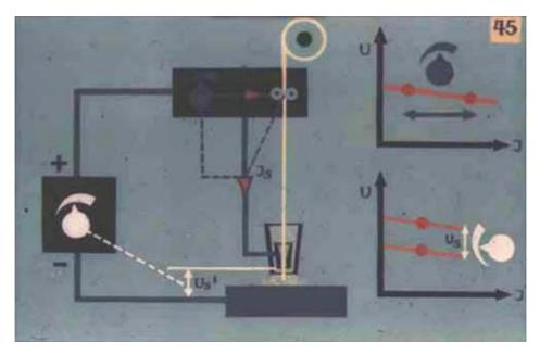
This slide shows where the most important  $CO_2$  welding parameters (U<sub>S</sub> and I<sub>S</sub>) have to be set.
