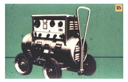
The following means are provided on the control panel of this motor-generator welding power source:
