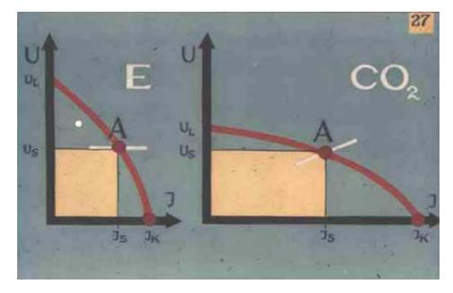
This slide shows the two basic forms of volt–amp output characteristic required for welding. Shown in the left and right parts of the slide, are respectively the drooping volt–ampere characteristic required for electric arc welding and the nearly flat characteristic used for gas metal–arc  $CO_2$  welding. Volt–ampere characteristics usually run from point U<sub>L</sub> (open–circuit voltage) to point I<sub>K</sub> (short–circuit current).
