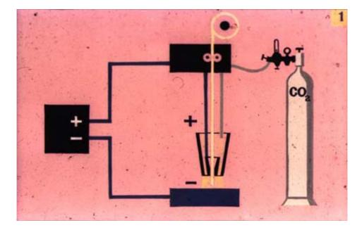
This slide shows the most essential components of a CO<sub>2</sub> gas–shielded arc welding unit and how they cooperate to enable operations of welding to be performed successfully. Metal–arc gas shielded welding with carbon dioxide shielding requires special weld power sources of which the operating principles will not be discussed until the fundamentals of electrical engineering have been described in detail.
