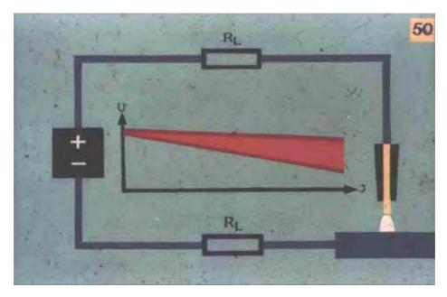
The length and cross section of the welding lead may have a substantial effect upon the  $CO_2$  welding operation.
