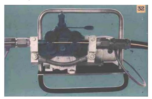
Slide no. 32 CO arc welding unit ZIS 707, side view
