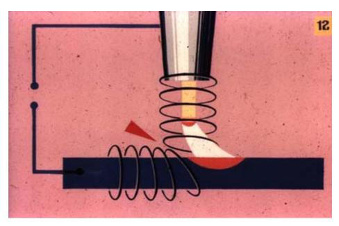
The formation of a magnetic field around a current–carrying conductor is known to have an adverse effect upon welding. This slide shows arc–blow–producing magnetic fields formed around the arc and work. The magnetic fields which are in a vertical relationship to each other cause the arc to be deflected in the direction of the arrow.
