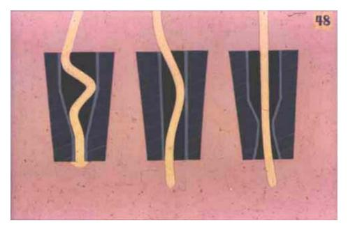
Contact tips have a decisive influence upon the weld operation. Extremely small tip bores result in the wire surface being worn off by friction, with the filler wire finally sticking fast in the tip, a phenomenon that is known as wire jam–up. In any case, heavy friction between the tip and filler metal wire will result in irregular wire feed which, in turn, causes the operation of welding to become quite irregular.
