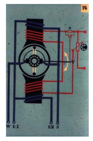
This slide shows the principle of construction of drooping and flat characteristic welding generators.
