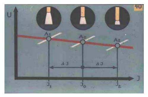
This slide shows the relations between volt–ampere and arc characteristics in  $CO_2$ –shielded welding. An average weld current ( $I_0$ ) is obtained for an average operating point ( $A_0$ ). A change in average arc length results in a longer length of the arc ( $A_1$ , with  $I_1$ ) or in a shorter length of the arc ( $A_2$  with  $I_2$ ).
