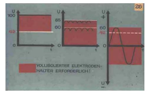
For welding in confined and moist spaces, it is necessary to set limits on the weld power source peak voltages.
