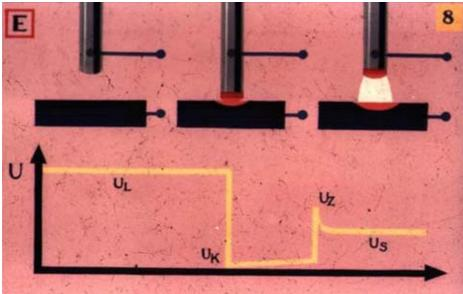
This slide shows the phases of starting the arc in electric arc welding. A distinction is generally made between no-load condition, ignition short-circuit, and arc.
