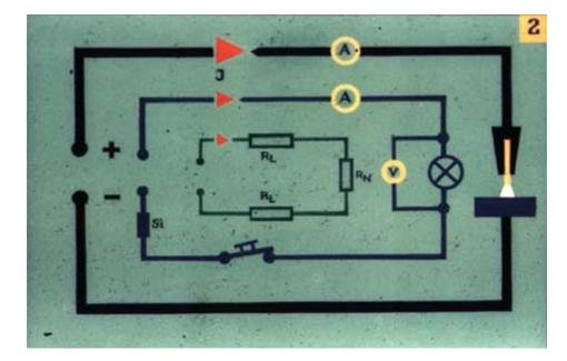
Slide no. 2 Comparison of basic and welding power circuits
