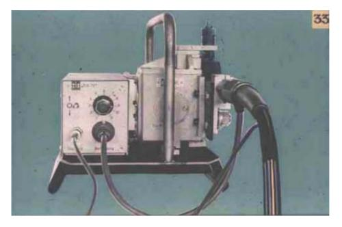
Slide no. 33 CO arc welding unit ZIS 707, front view
