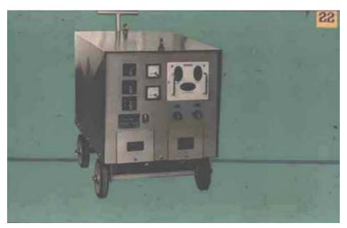
Slide no. 22 Welding rectifier RGS 315, general view
