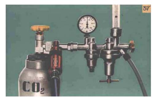
This slide shows the  $CO_2$  gas cylinder and no–freeze  $CO_2$  regulator. Adjusting means provided on the cylinder and regulator are marked in yellow.
