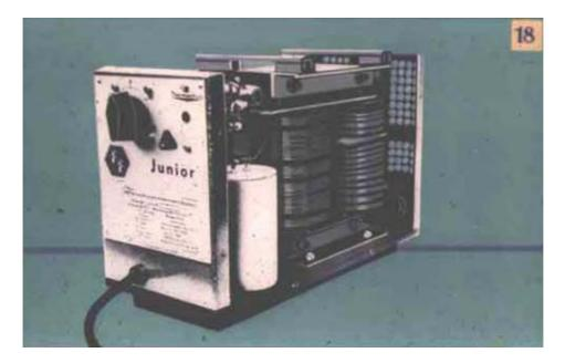
This slide is an interior view of the "Junior" welding type transformer, showing the primary and secondary windings of the transformer welding power source and the simplicity of mechanical construction thereof.
