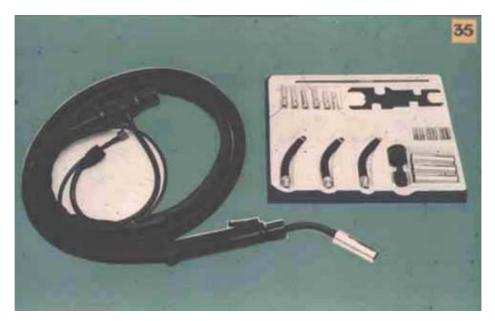
This slide shows an uncooled type of welding torch and torch accessories.
