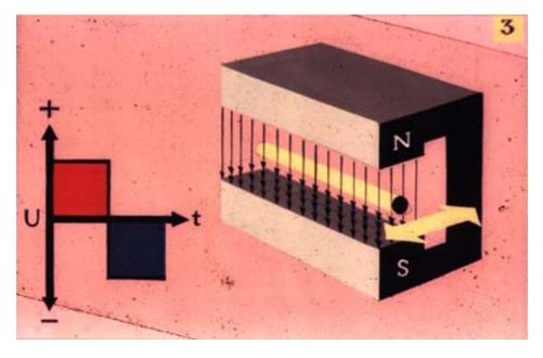
Voltage is the cause of current flow in the electric circuit. Therefore, it is not usually justifiable to use such terms as source of current or current supply source. This holds true especially for welding. There will be no flow of current until voltage is applied to an electric circuit. Well–known methods of voltage generation include
