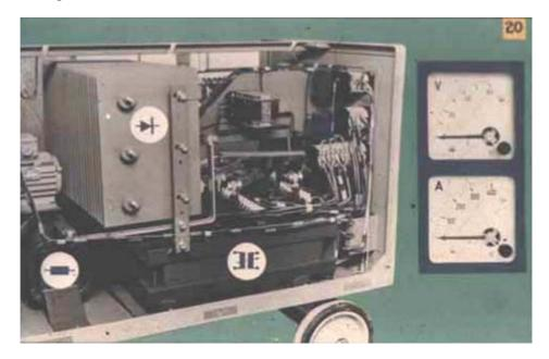
The principal components of this welding rectifier power source (namely, the transformer, rectifier, and reactor) are marked by symbols.
