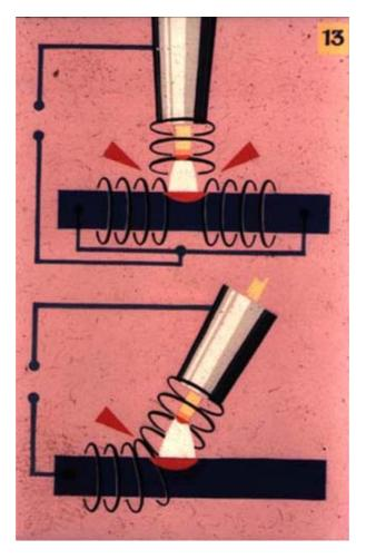
Connection of two parallel welding cables in opposite places is shown in the upper part of this slide, whereas the lower half of the slide illustrates the inclining of the weld torch as a possible way of combating arc blow.
