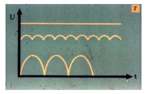
This slide shows different d–c voltage waveforms. D–C voltages of different waviness or ripple can be obtained depending on how voltage is generated.
