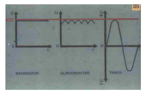
No-load voltages are limited to a maximum of 100 V for power sources for welding operations. It can be seen from this slide that these maximum values relate to the peak voltage. Be sure to point out that the voltmeters provided in welding power sources indicate r.m.s. (root mea square) values rather than peak voltages.
