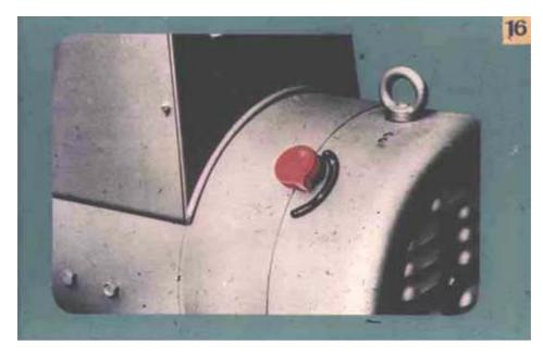
This motor–generator type welder, which has different volt–ampere output characteristics, can be used for open–arc,  $CO_2$ –shielded, and other welding processes.
