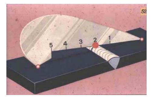
This slide shows that the same weld gage can be used to gage the reinforcement of a V groove weld. It is here, too, that three–point location is essential to correct gaging.
