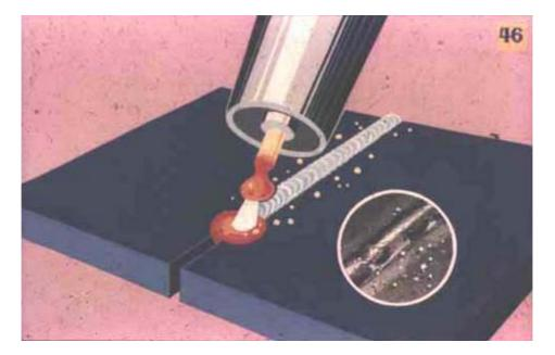
This slide shows the plate surface and the drop of metal when welding at too high a weld voltage.
