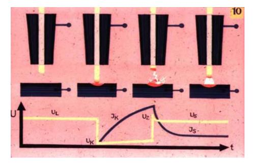
Starting of the  $CO_2$  welding arc differs from arc initiation as shown in slide no. 8 in that the open-circuit voltage is lower (with UL being roughly equal to  $U_s$ ) and the electrode need not be lifted off the work after ignition short-circuit.
