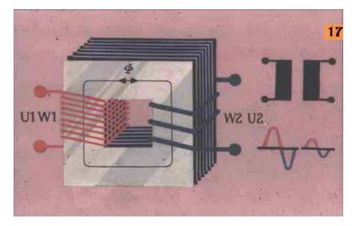
Slide no. 17 Welding transformer, principle of construction
