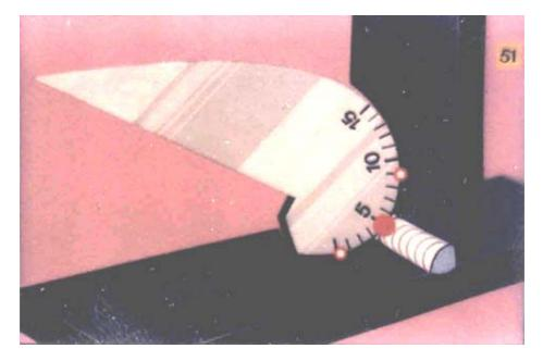
This slide shows how a weld gage can be used to determine the throat ("a") of a fillet weld. The fillet weld gage has been adjusted correctly when the conditions shown in the slide (three–point location) are satisfied.
