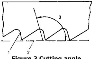
Figure 3 Cutting angle
