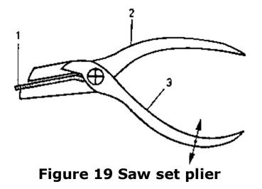
1 saw blade, 2 stationary lever of the plier, 3 movable lever which bends the saw tooth to the desired set width
