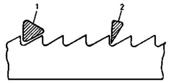
Figure 20 Cross-section of a file
