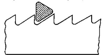
Figure 17 Filing out the tooth spaces
