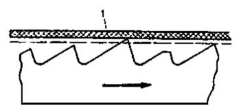
Figure 16 Adjusting the tooth points
