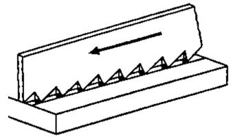
Figure 1 Cutting by saw teeth
