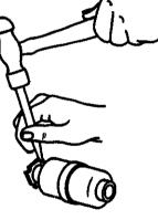
TIGHTEN MUFFLER LOCK NUT WITH HAMMER AND PUNCH
