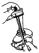
TIGHTEN ROD BOLTS TO SPECIFIED TORQUE
