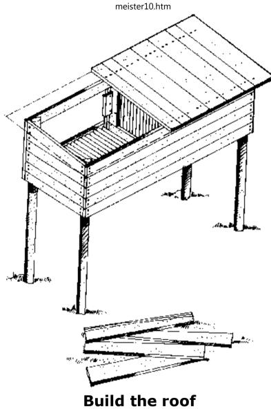
20 cover the roof with a piece of sheet metal or pieces of tin cut from cans
