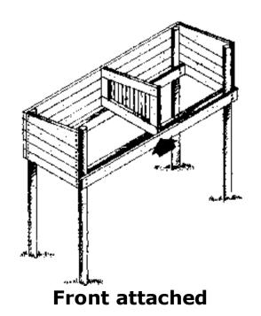
12 when the board is in place, make sure that the wall in the centre is straight and fasten the front of the wall to the board (see arrow)
