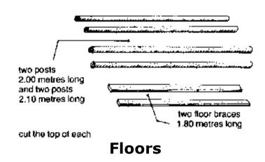
2 cut the top of each of the floor braces as shown to keep the rabbit droppings from collecting on top of the boards
