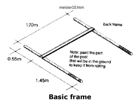
4 build the basic frames for the pens one frame for the back and one frame for the front, as shown above and below
