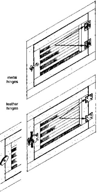
Using metal hinges or strips of leather
