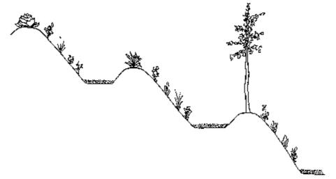
digging trenches along level contours and form elevated ridges for tree planting
