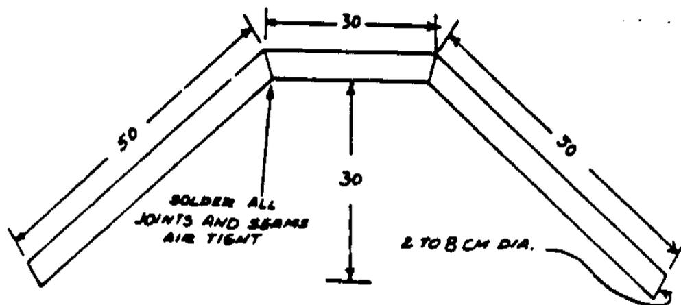
**Figure 1: Siphon Tube for Flood and Furrow Irrigation**
