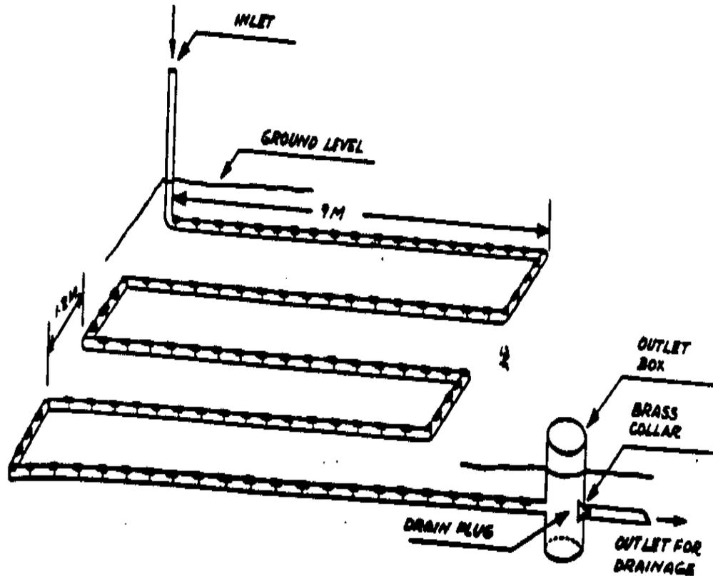
**Figure 3: Simple Drip Irrigation System**
