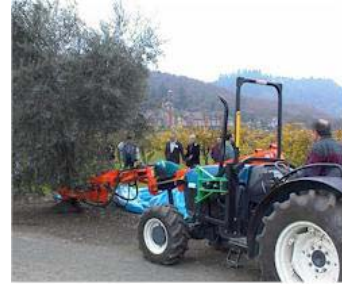
Tractor mounted shaker
