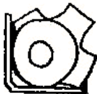
STANDARD BICYCLE BOTTOM BRACKET AND SPINDLE ASSEMBLY BRAZED TO LATERAL ADJUSTMENT INTERMEDIARY MILD STEEL ANGLE, 50X50X6X67mm LONG
