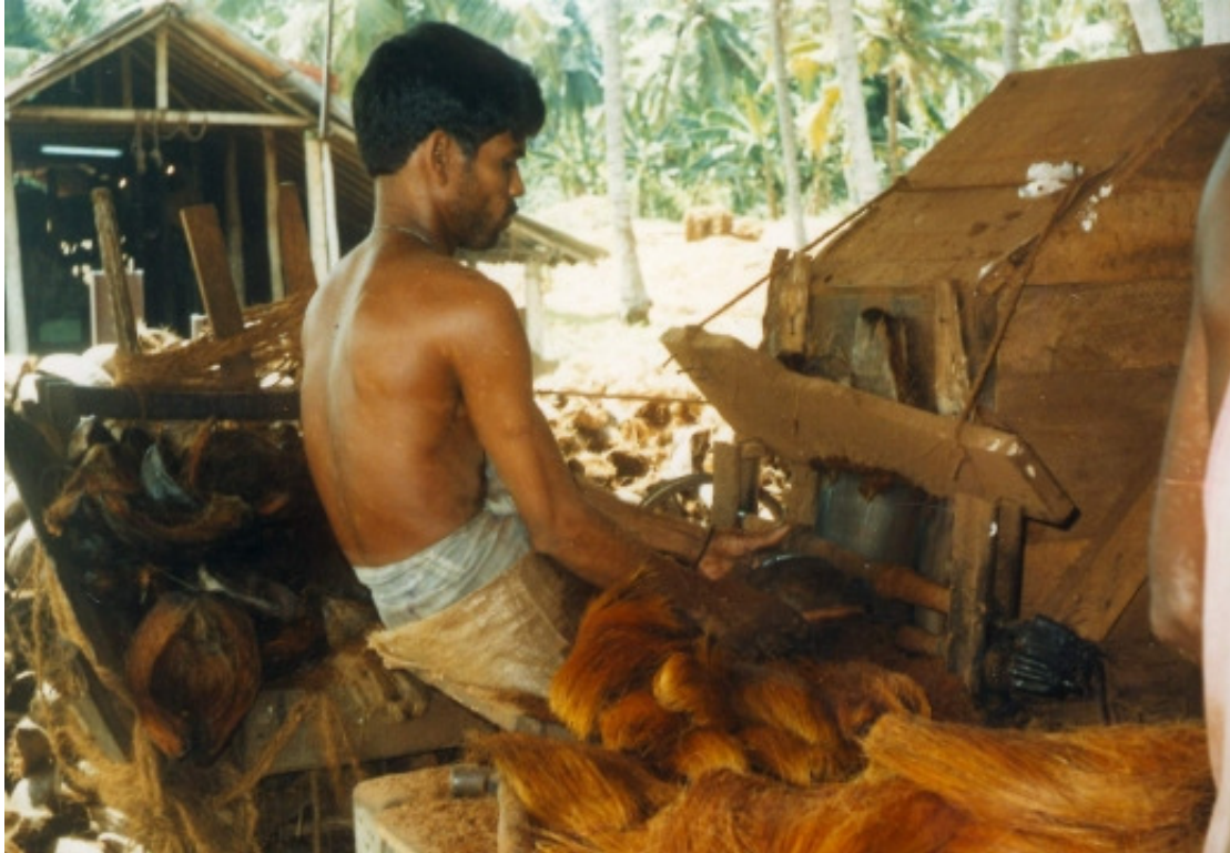
Figure 20a: Mechanical extraction of the coconut husk
