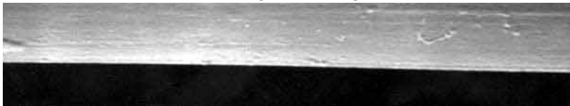
5. A brin of degummed cocoon bave (5,000 times by SEM)
