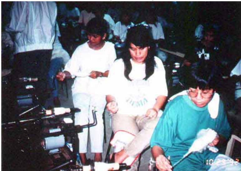
30. Hand-spun silk reeling machine (from floss silk)
