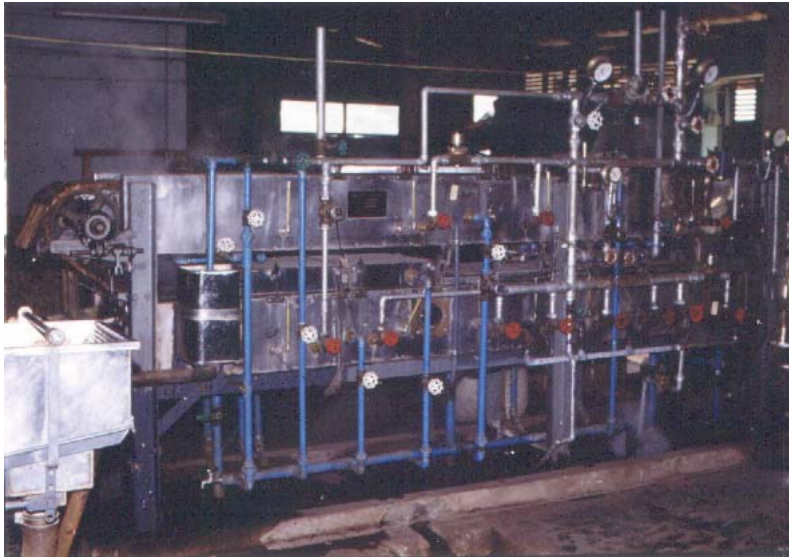
16. Cocoon cooking machine (1 basket circulating type)
