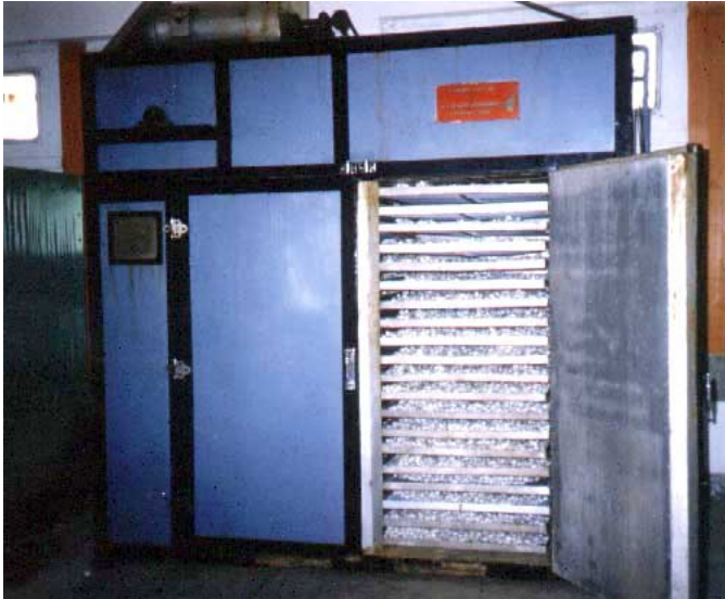
10. Cabinet type cocoon dryer (Shelf-carrier type)
