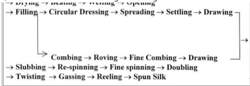
Figure 17. Spun silk manufacturing process.
