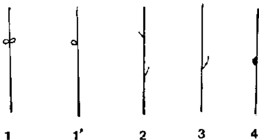
Figure 2 – Neatness defects (1) (1') Loop (2) Hairiness (3) Split-ends (4) Nibs
