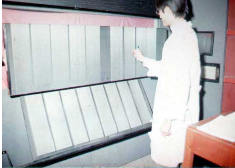
38. Seriplane inspection for cleanness and neatness
