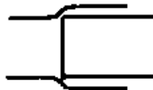
Drain sleeve connection
