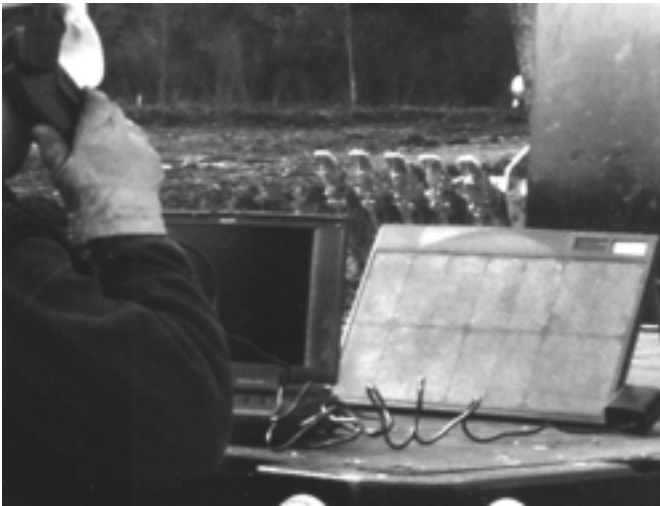
SC8501 Portable Energy System powering a cellular telephone and laptop computer in a remote construction site
