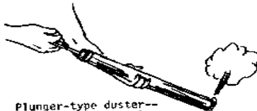
Plunger-type duster-- Looks like a bicycle pump
