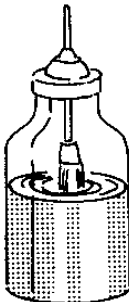
FIGURE 3. A DISPENSER CAN BE MADE BY CUTTING A HOLE IN THE COVER LARGE ENOUGH FOR THE HANDLE OF A 2.5 CM. BRUSH. THE DISPENSER MUST BE AIRTIGHT SO THAT THE CEM
