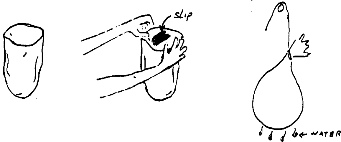
Figure 20. Drying Clay in a Cloth Bag
