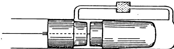
Phase 3: Piston remaining at top dead center. Displacer has shifted gas through cooler, regenerator, and heater into hot space.
