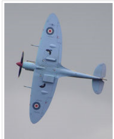
The elliptical wing and tail units are shown to good effect in this photograph of a Spitfire Mk VR which also shows
