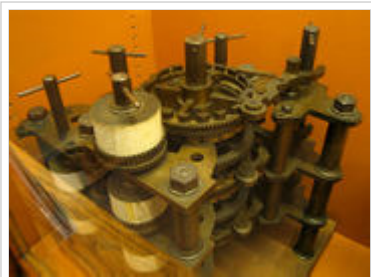
Part of Charles Babbage's Difference Engine including the addition and carry mechanisms
