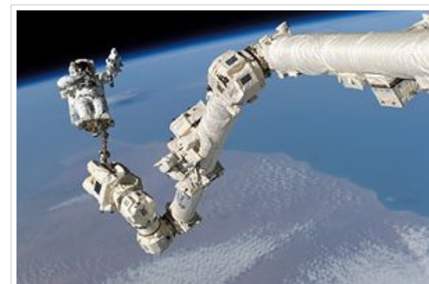
The Canadarm2 robotic manipulator on the International Space Station is operated by controlling the angles of its joints. Calculating the final position of the astronaut at the end of the arm requires repeated use of the trigonometric functions of those angles.
