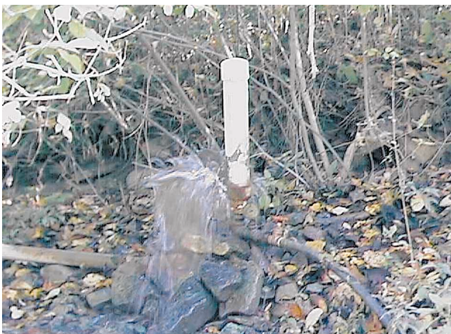
Scott Lee's ram pump in operation.
