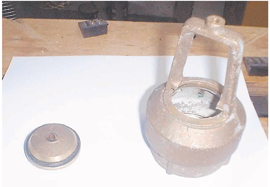
The foot valve on its way to becoming the waste valve—the stem is cut off the valve disc and the lower crosspiece has been cut away from the casting.
