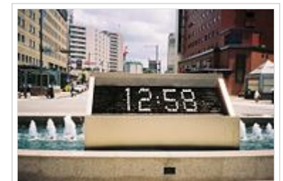
Digital clock outside Kanazawa Station displaying the time by controlling valves on a fountain
