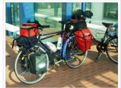
Touring bicycle equipped with head lamp, pump, rear rack, fenders/mud-guards, water bottles and cages, and numerous saddle-bags.
