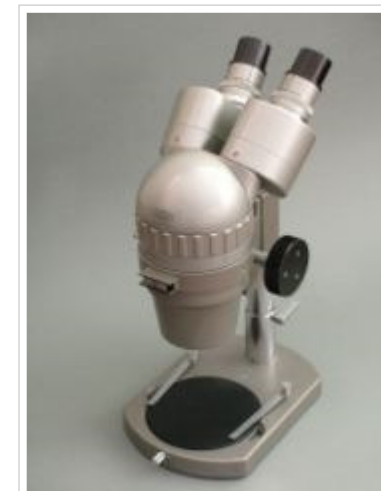
A stereo microscope is often used for lower-power magnification on large subjects.
