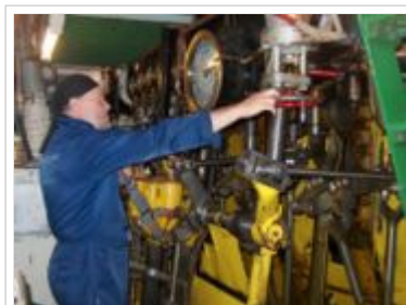
SS Ukkopekka triple expansion steam engine
