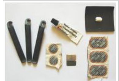
Puncture repair kit with tire levers, sandpaper to clean off an area of the inner tube around the puncture, a tube of rubber solution (vulcanising fluid), round and oval patches, a metal grater and piece of chalk to make chalk powder (to dust over excess rubber solution). Kits often also include a wax crayon to mark the puncture location.
