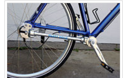
A bicycle with shaft drive instead of a chain
