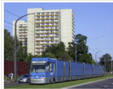
Volkswagen Cargo-Tram in Dresden, Germany on a section of grassed track. It delivers parts to the Transparent Factory
