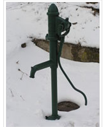
Hand-operated, reciprocating, positive displacement, water pump in Košice- Ľahanovce, Slovakia (walking beam pump).
