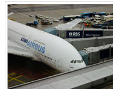
A380 being serviced by three separate jetways at Frankfurt Airport; two for the main deck and one for the upper deck.
