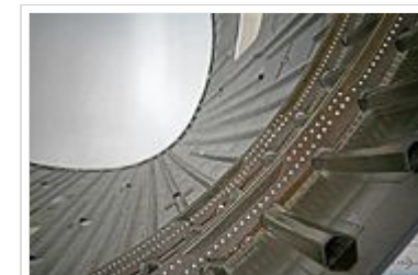
Disassembled fuselage section of the Boeing 787 Dreamliner
