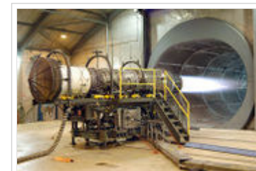
A Pratt & Whitney F100 turbofan engine for the F-15 Eagle and the F-16 Falcon is tested at Robins Air Force Base, Georgia, USA. The tunnel behind the engine muffles noise and allows exhaust to escape
