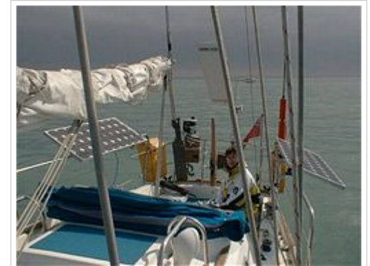
The solar panels on this small yacht at sea can charge the 12 volt batteries at up to 9 amperes in full, direct sunlight.
