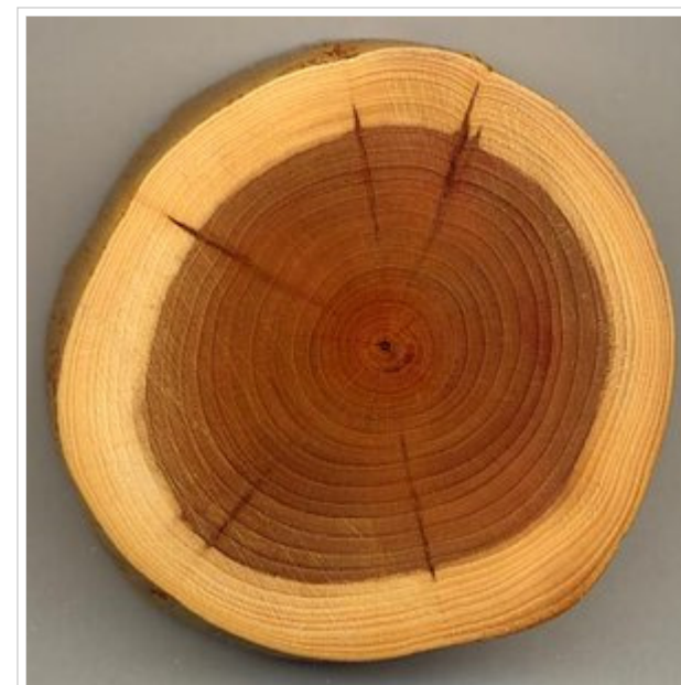
A section of a Yew branch showing 27 annual growth rings, pale sapwood and dark heartwood, and pith (centre dark spot). The dark radial lines are small knots.
