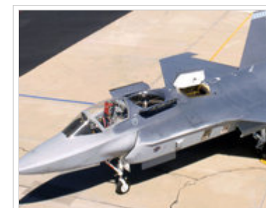
X-35B lift fan; the VTOL propulsion system is designed and manufactured by Rolls-Royce plc
