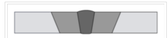
The cross-section of a welded butt joint, with the darkest gray representing the weld or fusion zone, the medium gray the heat-affected zone, and the lightest gray the base material.
