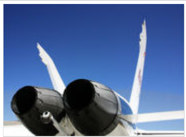
Variable Exhaust Nozzle, on the GE F404-400 low-bypass turbofan installed on a Boeing F/A-18 Hornet
