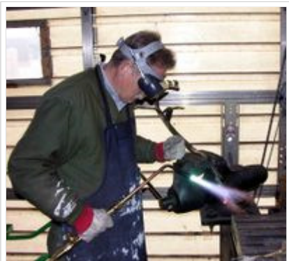
Gas welding a steel armature using the oxy-acetylene process.
