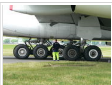
The A380's 20-wheel main landing gear
