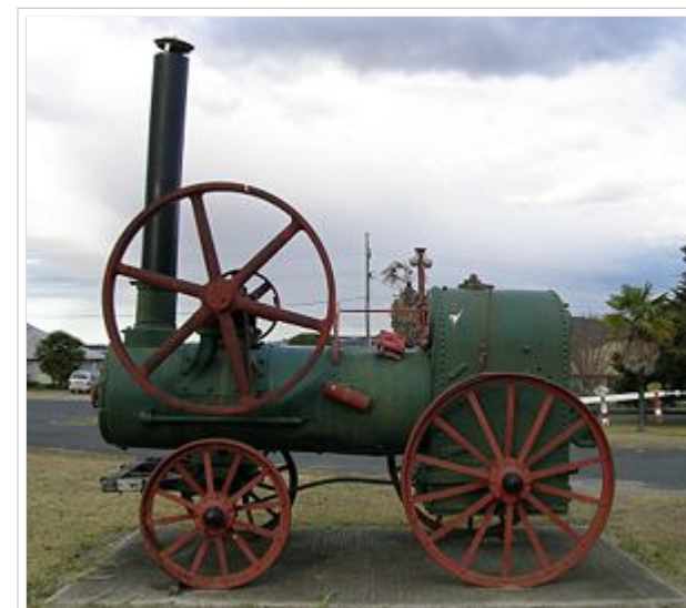
'Preserved' (but incomplete) portable engine, Tenterfield, NSW – an example of a mobile steam engine
