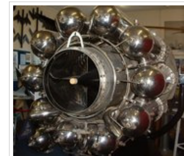
The Whittle W.2/700 engine flew in the Gloster E.28/39, the first British aircraft to fly with a turbojet engine, and the Gloster Meteor
