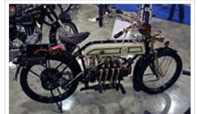
A 1913 Fabrique National in-line four with shaft drive from Belgium
