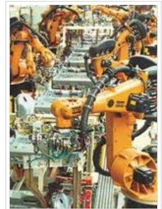
Industrial robots perform repetitive tasks, such as assembling vehicles.
