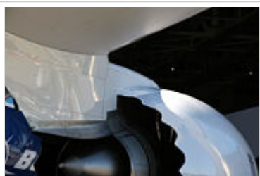
The engine pods on the 787 feature chevron edges to reduce noise.
