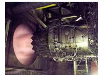
A Pratt and Whitney F135 engine undergoes altitude testing at the Arnold Engineering Development Centre.
