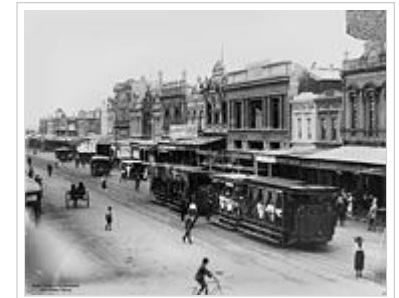
Steam trams in Rockhampton, Queensland - note the small boiler at the front of the leading tram.
