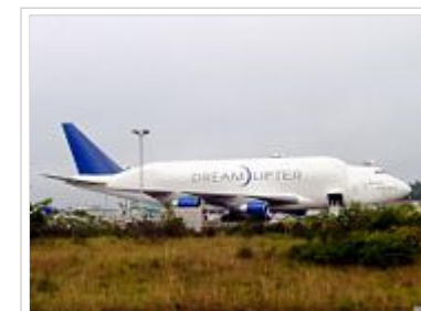
Three Dreamlifter 747s are used to transport 787 fuselage sections.
