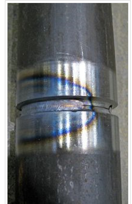
The blue area results from oxidation at a corresponding temperature of 600 °F (316 °C). This is an accurate way to identify temperature, but does not represent the HAZ width. The HAZ is the narrow area that immediately surrounds the welded base metal.
