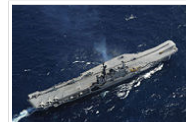
India's light carrier INS Viraat , formerly HMS Hermes , purchased from the British, after INS Vikrant shows another example of the ski jump.
