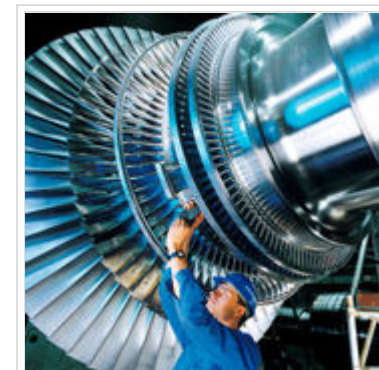
A rotor of a modern steam turbine , used in a power plant
