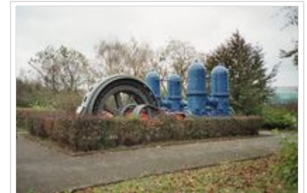
A large, electrically driven pump (electropump) for waterworks near the Hengsteysee, Germany.
