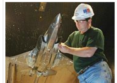
An F-35 wind tunnel testing model in the Arnold Engineering Development Centre's 16-foot transonic wind tunnel
