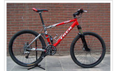
This mountain bicycle features oversized tires, a full-suspension frame, two disc brakes and handlebars oriented perpendicular to the bike's axis
