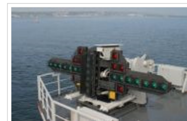
Landing optics of Charles de Gaulle , note that this system is of the later Fresnel lens design.
