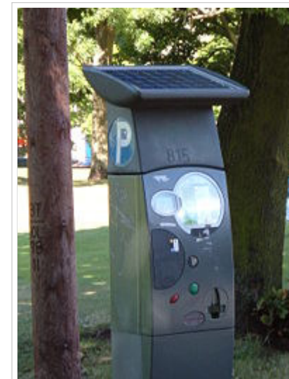
A solar panel on top of a parking meter. Note that this particular installation is shaded, and may not perform as desired.
