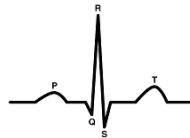
Figure 1.3: An example of the typical shape and location of the various components of an ECG signal.
