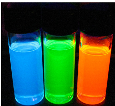
Figure 8.1: Picture of cadmium selenide (CdSe) quantum dots, dissolved in toluene, fluorescing brightly, as they are exposed to an ultraviolet lamp, in three noticeable different colors (blue \sim 481 nm, green \sim 520 nm, and orange \sim 612 nm) due to the quantum dots' bandgap (and thus the wavelength of emitted light) depends strongly on the particle size; the smaller the dot, the shorter the emitted wavelength of light. The "blue" quantum dots have the smallest particle size, the "green" dots are slightly larger, and the "orange" dots are the largest.
