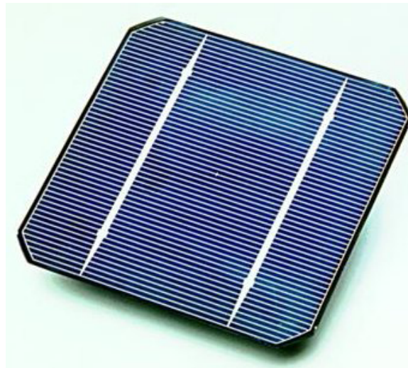
Figure 2.36: A solar cell showing the blue tint due to the AR coating.
