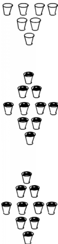
Figure 1.4: Silicon, with first two bands full and the next empty.
