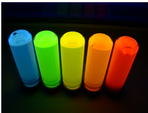
Figure 8.4: Fluorescing CdSe quantum dots synthesized in a heat transfer liquid of different sizes (M. S. Wong, Rice University).
