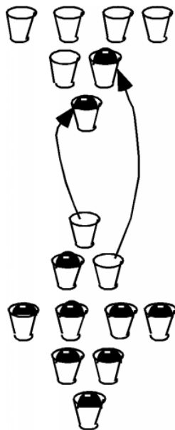
Figure 1.6: Thermal excitation of electrons across the band gap.
