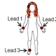
Figure 2.2: Lead 1 is attached to the right wrist, Lead 2 to the left wrist and Lead 3 is attached to the right ankle as a ground electrode.
