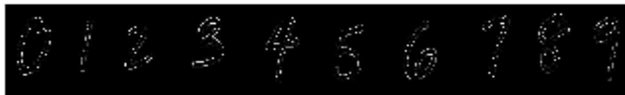
Figure 6.5: Result of edge detection with sobel operator.
