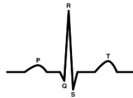
Figure 2.3: An example of the typical shape and location of the various components of an ECG signal.
