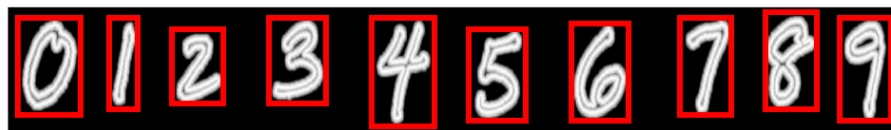
Figure 6.7: Connected regions are identified by ‘boundingbox’
