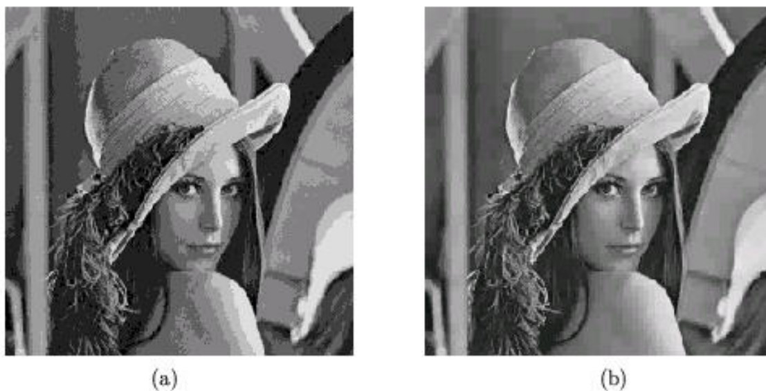
Figure 2.13: Images reconstructed from (a) the original Lenna, and (b) the 4-level Haar transform, each quantised with Q_{\text{step}} = 30 . The rms error of (a) = 8.6219, and of (b) = 5.8781.
