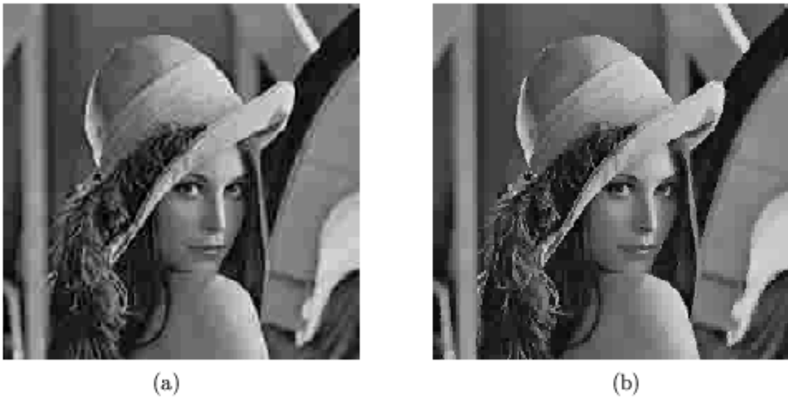
Figure 4.19: Reconstructions after coding using the 8 \times 8 DCT (a) with Q_{\text{step}} = 5Q_{\text{lum}} , and (b) using the Haar transform with Q_{\text{step}} from Table 4.2.
