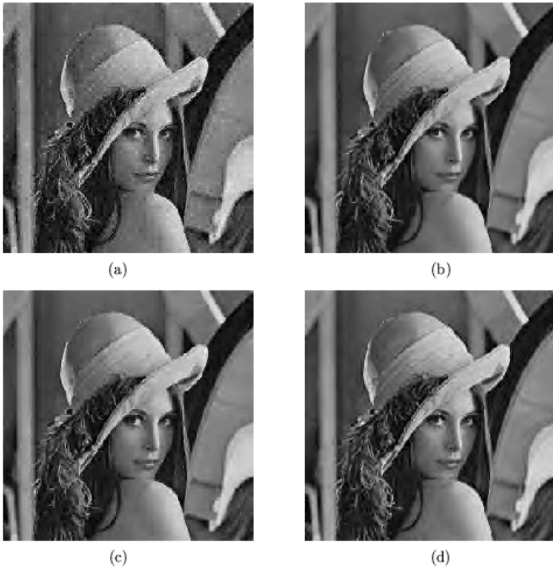
Figure 4.20: Reconstructions after coding using Q_{\text{step}} from Table 4.2 with (a) the LeGall 3,5-tap filters, (b) the inverse-LeGall 5,3-tap filters, (c) the near-balanced 5,7-tap filters, and (d) the near-balanced 13,19-tap filters.
