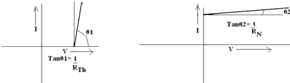
Figure 3 Real Voltage Source and Real Current Source I-V characteristics.
