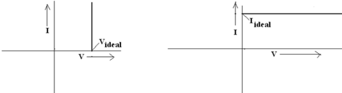
Figure 2 Ideal Voltage Source and Ideal Current Source I-V characteristics.
