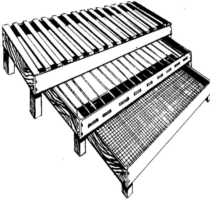
*FIGURE 2. THE THREE BEDS ARE MADE TO FIT ONE UNDER THE OTHER, SAVING ON SPACE WHEN NOT IN USE. THREE DIFFERENT KINDS OF SPRING ARE SHOWN: WOOD ON THE LARGEST BED, ROPE ON THE MIDDLE-SIZE BED AND CHICKEN WIRE ON THE SMALLEST BED.*
