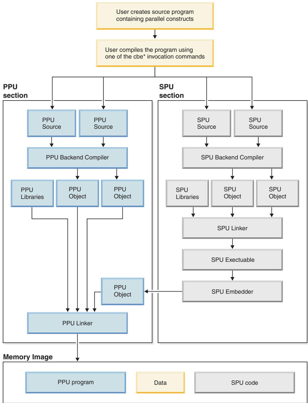
For some background information on how the single-source compiler works to compile code optimized specifically for use on the Cell Broadband Engine architecture, see the "Generation of Parallel Code" section in the article "Using advanced compiler technology to exploit the performance of the Cell Broadband Engine architecture" which can be found online at <http://www.research.ibm.com/journal/sj/451/eichenberger.html>.
