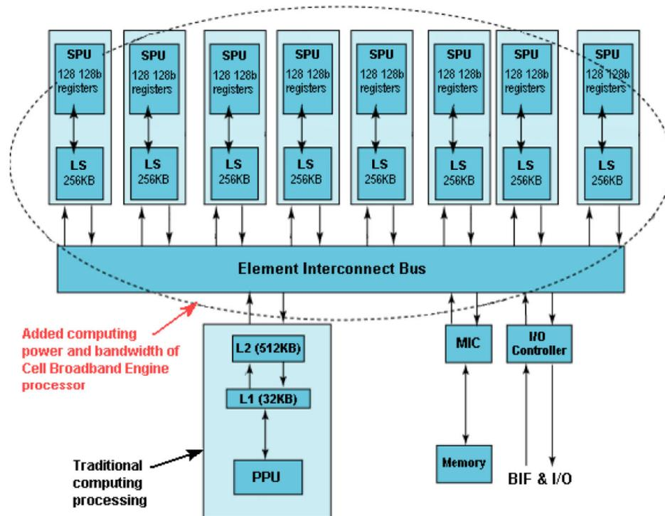
In operation, the PPU runs the operating system and performs high-level application control, while the SPUs divide and perform an application's computational work between them.
