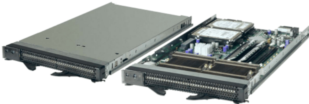
Figure 3.3: View of an HS20 Blade Server
