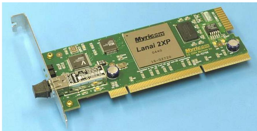
One-port NICs: "D card" (225MHz) & "F card" (333MHz)
