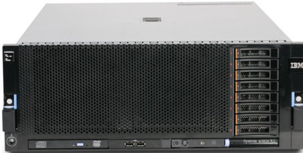
Figure 2. IBM System x3850 X5 Server
