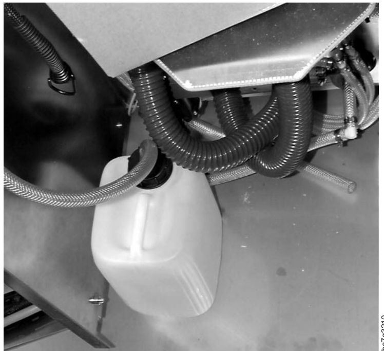
Figure 273. Condensation Water Reservoir
