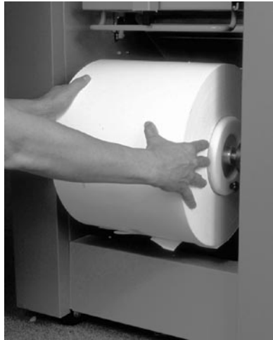
Figure 242. Pushing Paper Roll into Place
