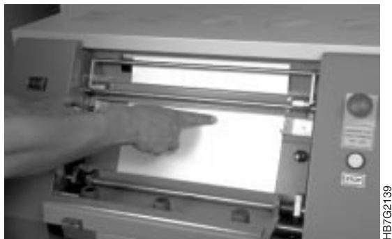
Figure 216. Rubbing the Paper Splice
