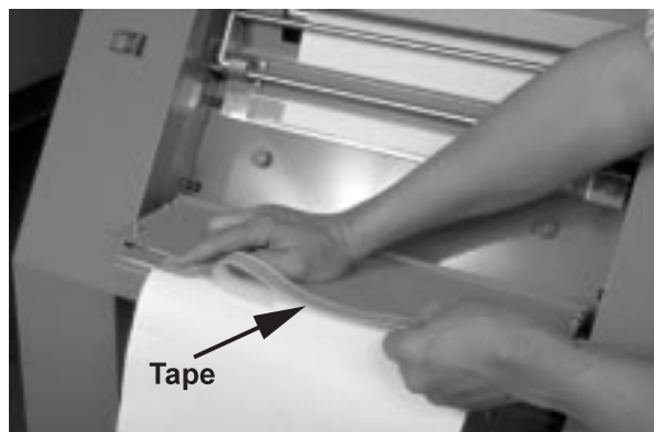
Figure 208. Attaching the Splicing Tape
