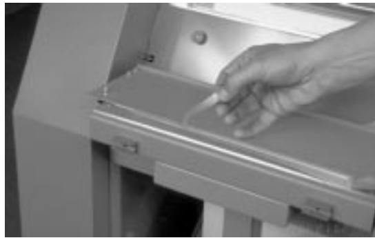
Figure 214. Pulling the Backing from the Splicing Tape
