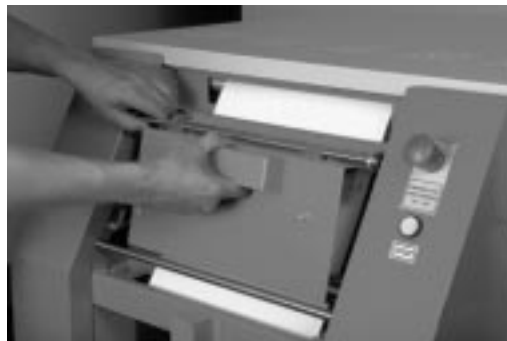
Figure 237. Returning Splicing Table to its Normal Position
