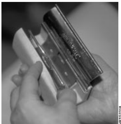
Figure 329. Insert Paper in Left Side of Polishing Pad
