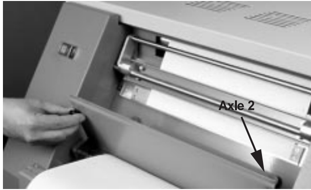
Figure 293. Inserting the Paper Between the Splicing Table and the Plate
