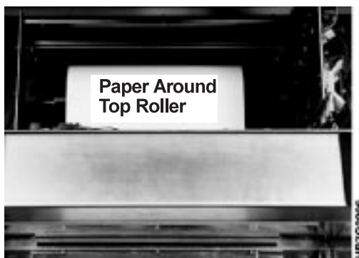
Figure 311. Threading the Paper Around the Top Roller
