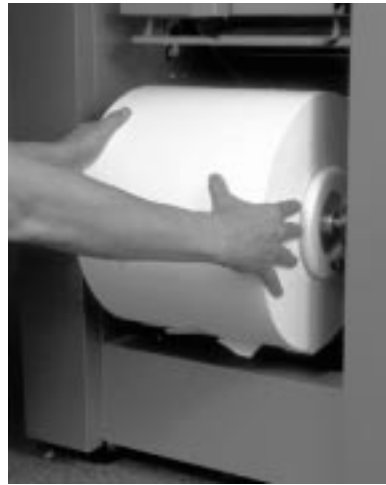
Figure 201. Pushing Paper Roll into Place
