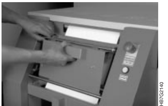
Figure 217. Returning Splicing Table to its Normal Position
