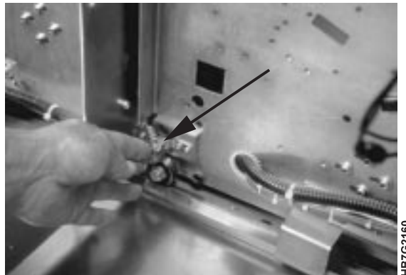
Figure 269. Unlatching Bottom of X and Y Tower
