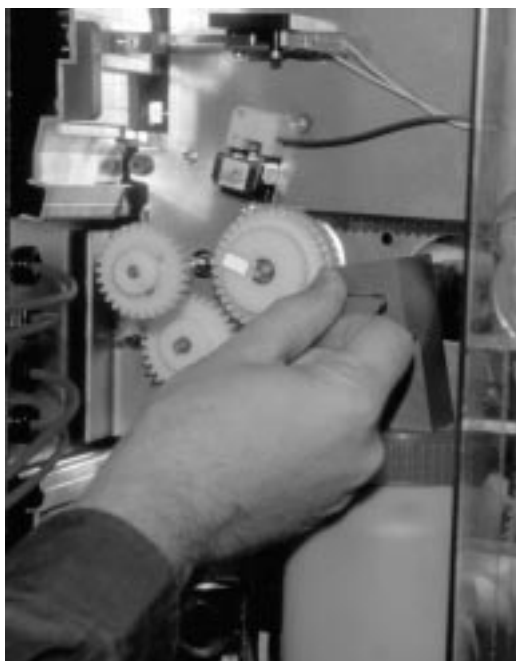
Figure 266. Rotating the Waste Bottle Handle
