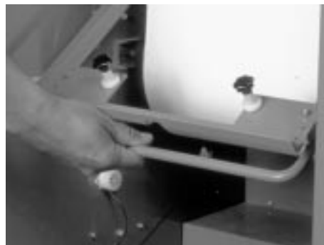
Figure 202. Lifting the Paper Supply Brake Lever
