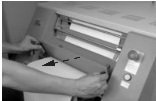
Figure 205. Closing the Clamping Plate
