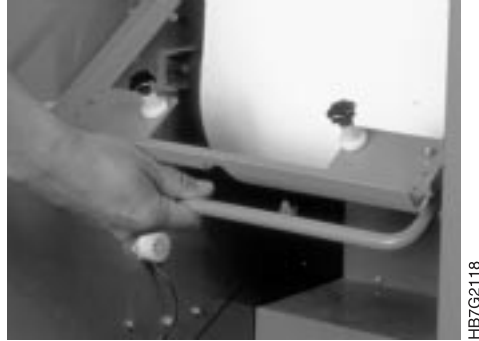
Figure 234. Lifting the Paper Supply Brake Lever
